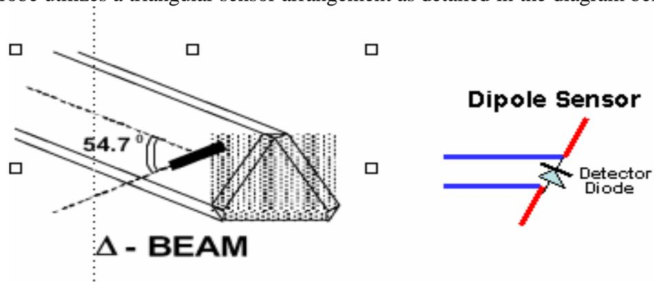
SAR is assessed with a calibrated probe which moves at a default height of 5mm from the center of the diode, which is mounted to the sensor, to the phantom surface (in the Z Axis). The 5mm offset height has been selected so as to minimize any resultant boundary effect due to the probe being in close proximity to the phantom surface.
