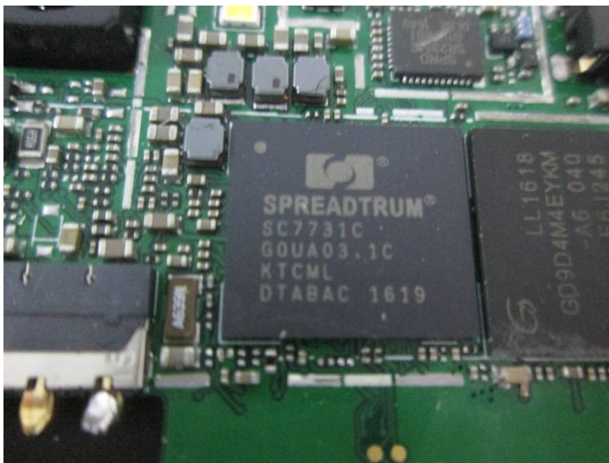
EUT –Main IC View
