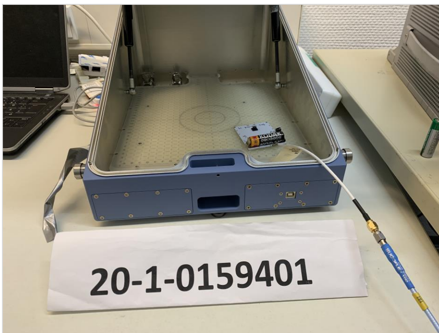
Photograph 6: EUT Setup in the radio lab 2, open box view
