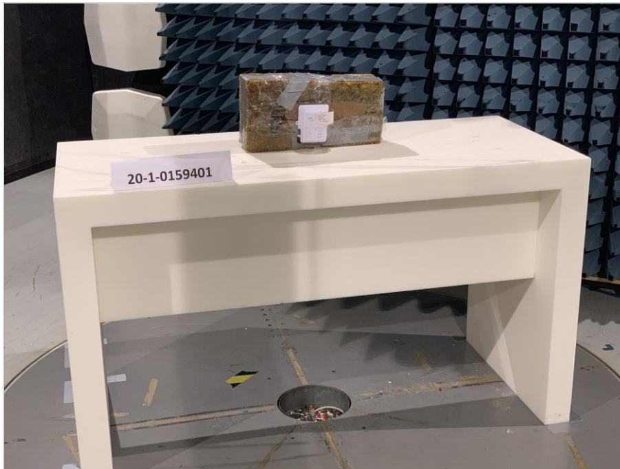
Photograph 1: EUT Test Setup in the anechoic chamber, Radiated interference field strength, close view
