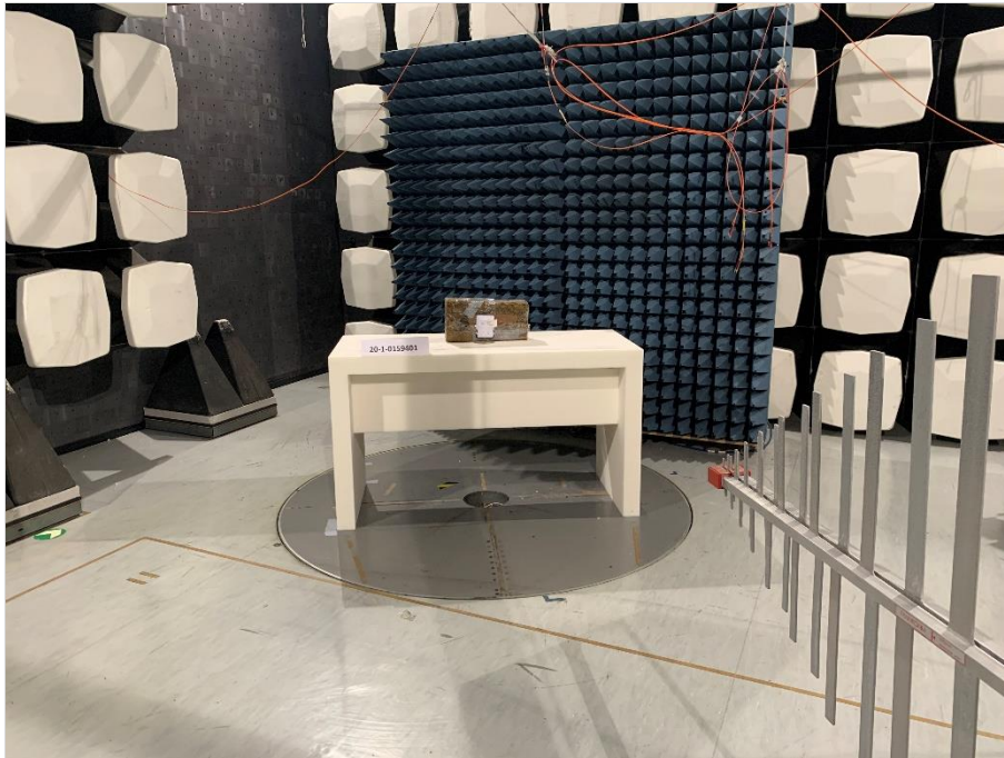
Photograph 3: EUT Test Setup in the anechoic chamber, Radiated interference field strength 30 MHz – 1 GHz, overview
