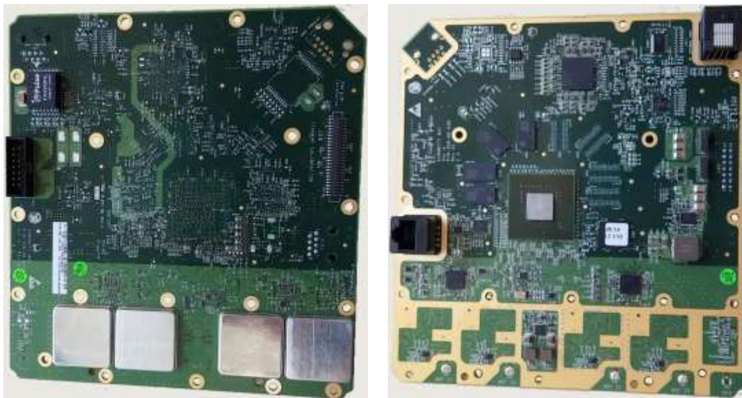
Figure 2: AU540 eNB B41 – both sides
