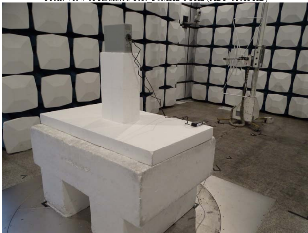
Front View of Radiated Test 30MHz-1GHz (ADP-65JH HB)
