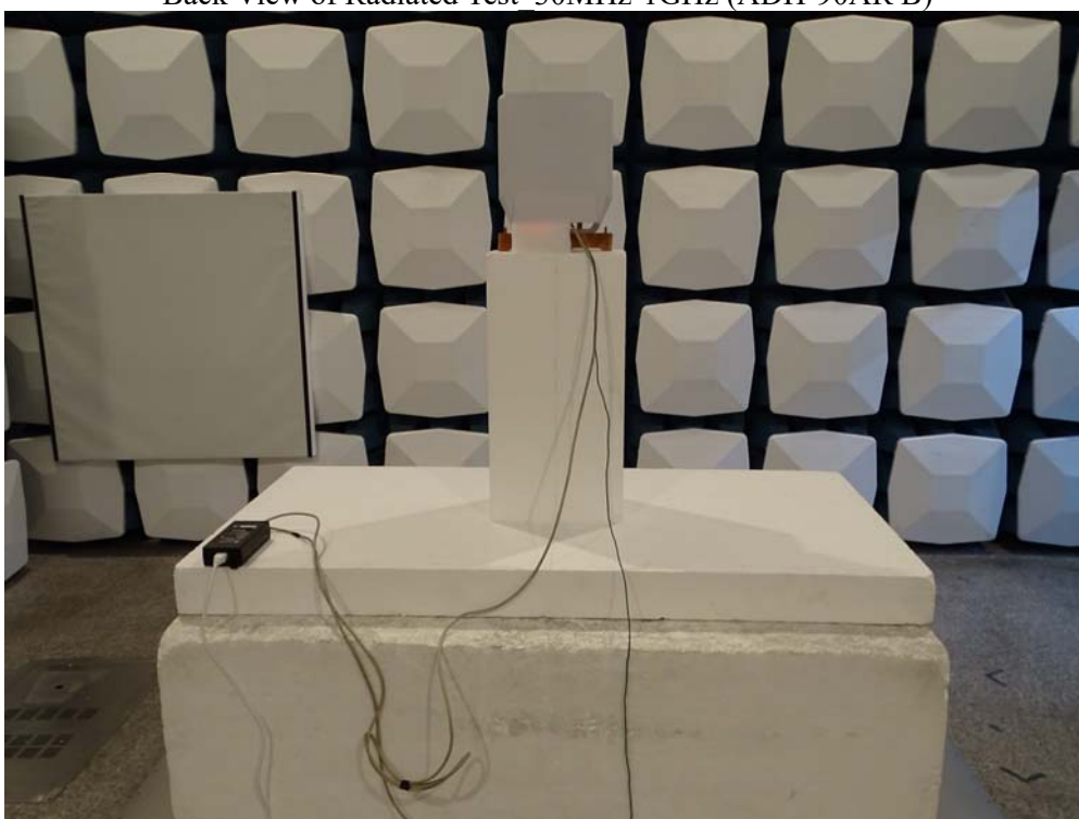
Back View of Radiated Test 30MHz-1GHz (ADH-90AR B)
