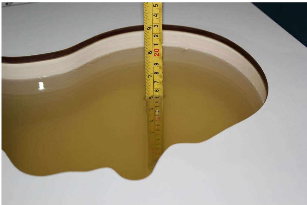
Picture 7-6: Liquid depth in the Head Phantom(2550MHz)
