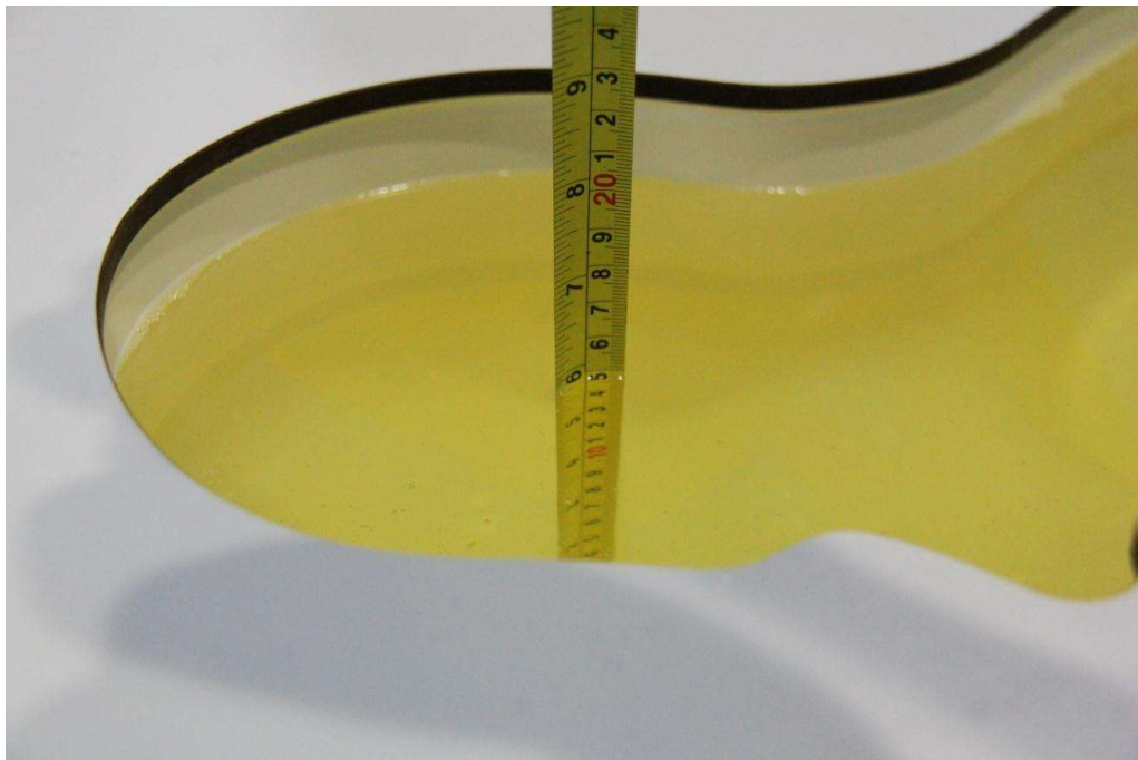
Picture 7-5: Liquid depth in the Head Phantom(2450MHz)
