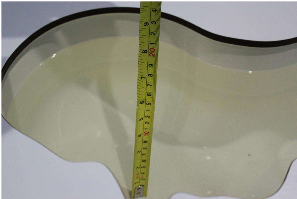
Picture 7-7: Liquid depth in the Head Phantom(5GHz)
