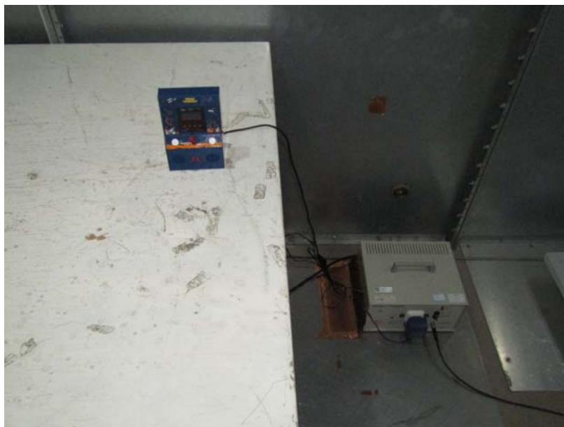
Measurement of Conducted Emission Test Set Up
