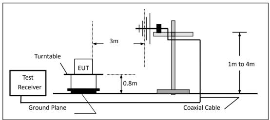
(c) For radiated emissions above 1000MHz
