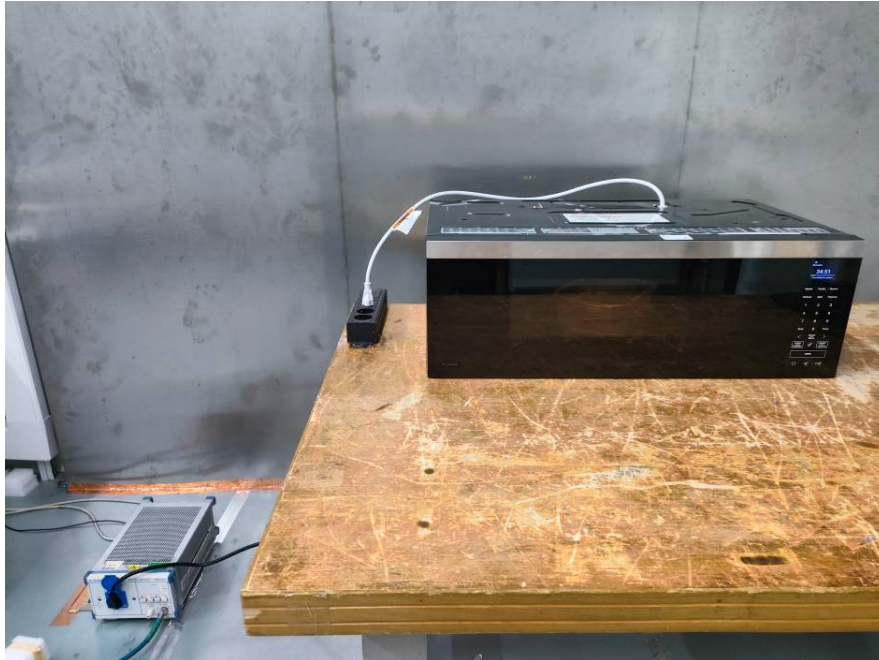
Conducted Emissions Side View
