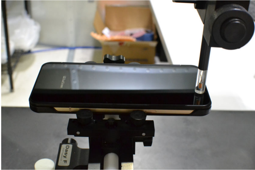
Figure 16-3 Test Setup for Wireless Device with Dual Display - Closed
