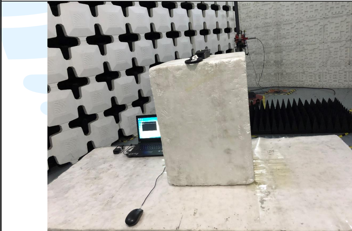
Radiated emission Test Setup (Above 1 GHz)
