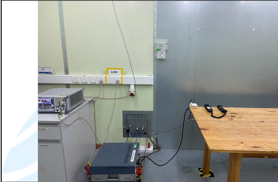
Conducted Emission Test Setup
