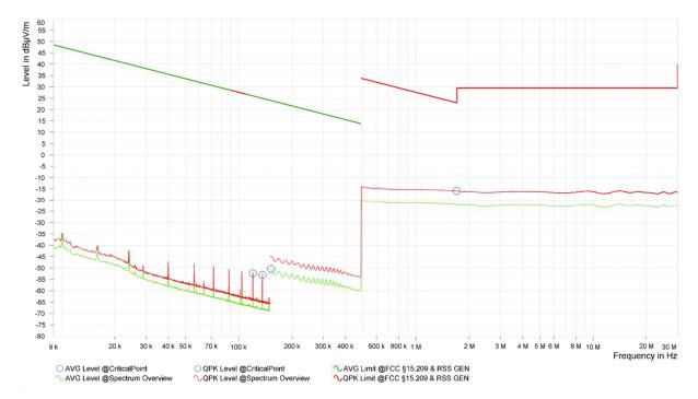
Spurious emissions from 9 kHz to 30 MHz (operation mode 2, position 1):
