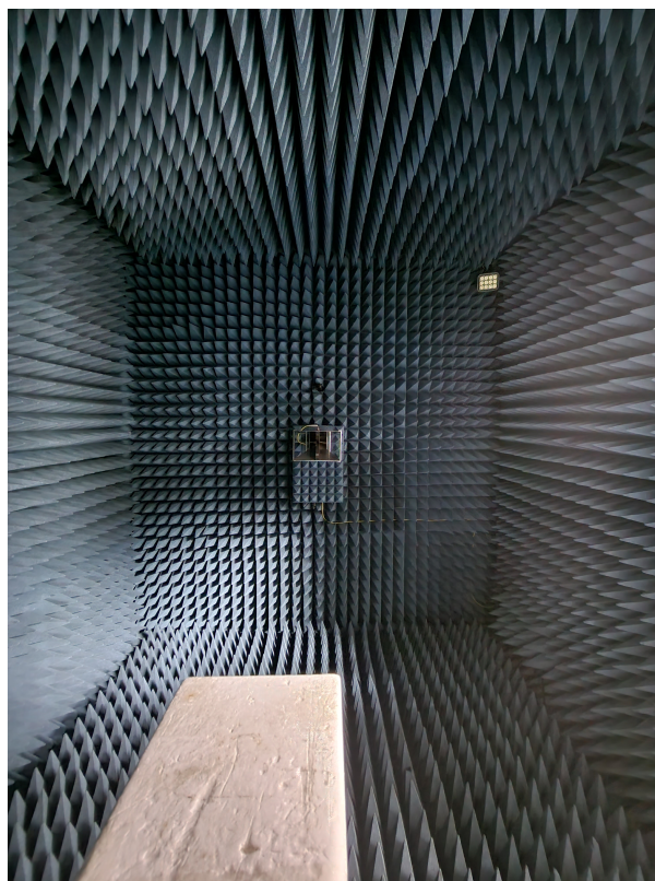
Figure 2: Geometry of Anechoic Chamber for Radiation patterns.
