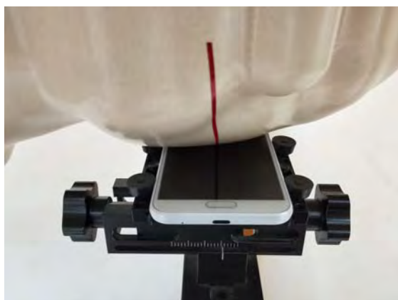
Fig.5 Left Head Section / Cheek-Touch Position
