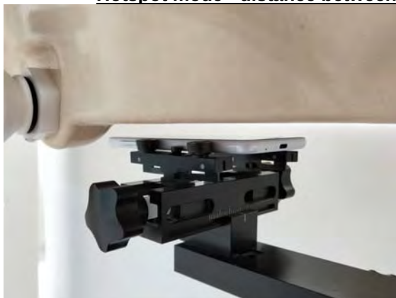
Fig.9 EUT Front side to flat phantom
