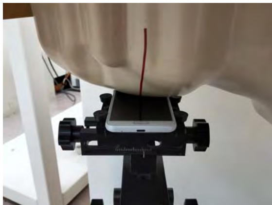
Fig.3 Right Head Section / Cheek-Touch Position
