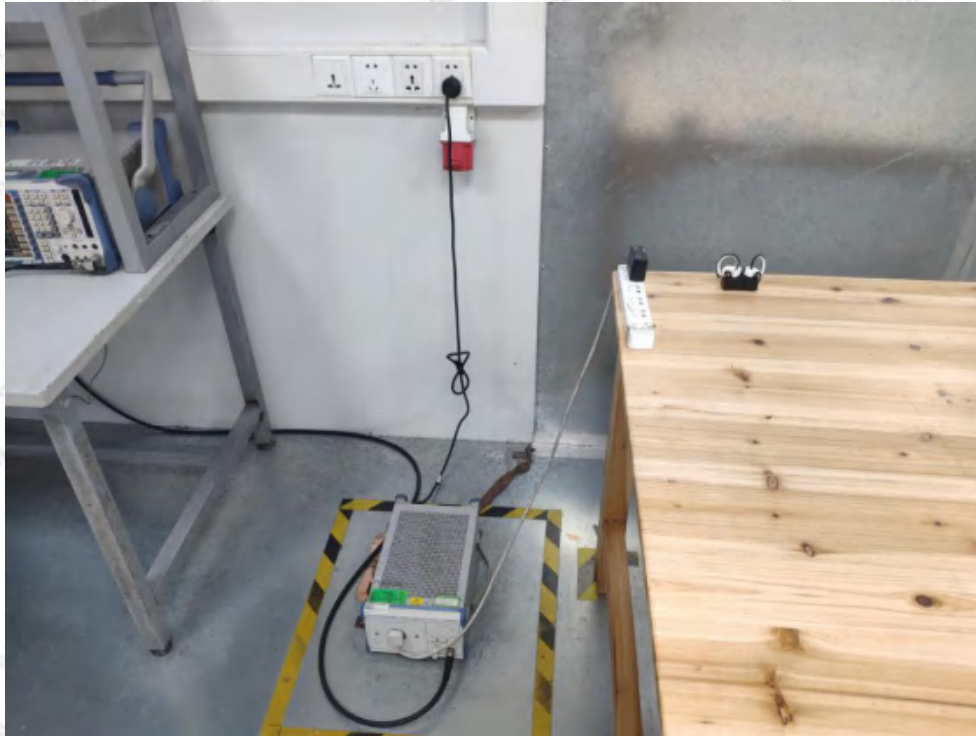
Photo of Conducted Emission Measurement
