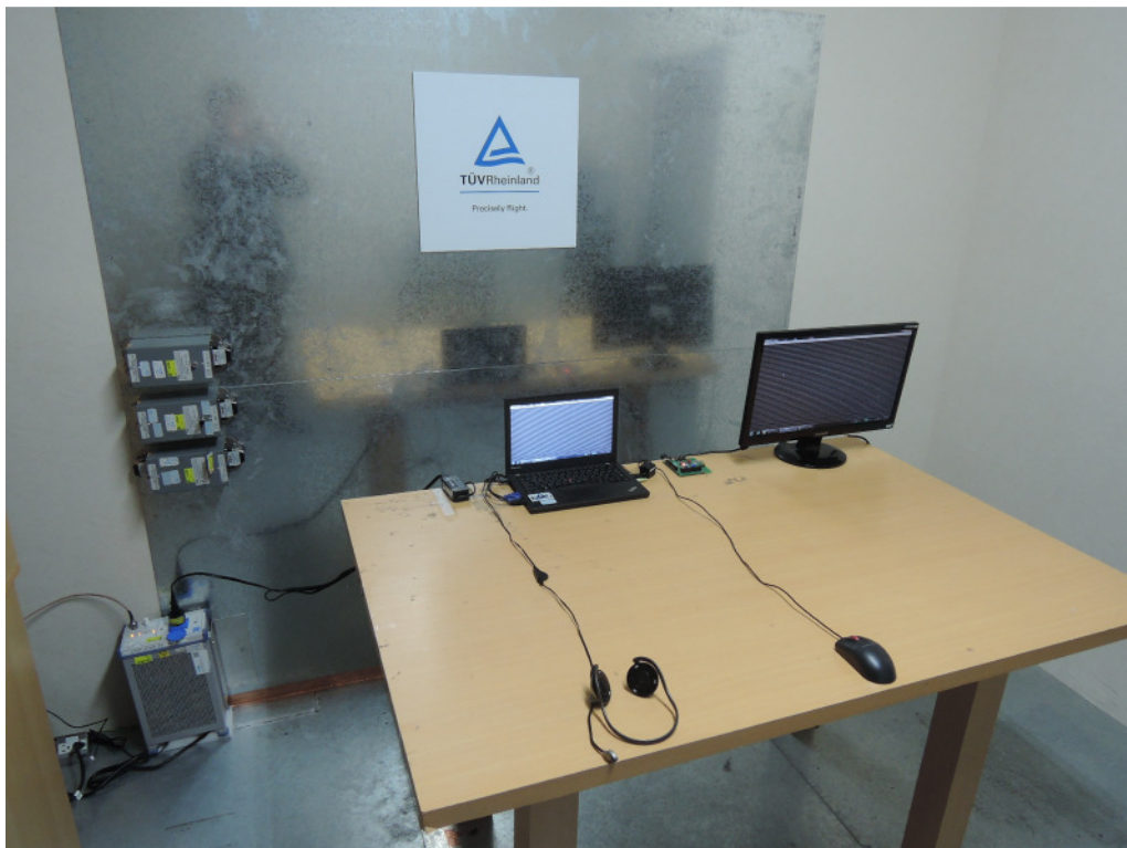
Photograph 6: Set-up for for Mains Conducted testing Front
