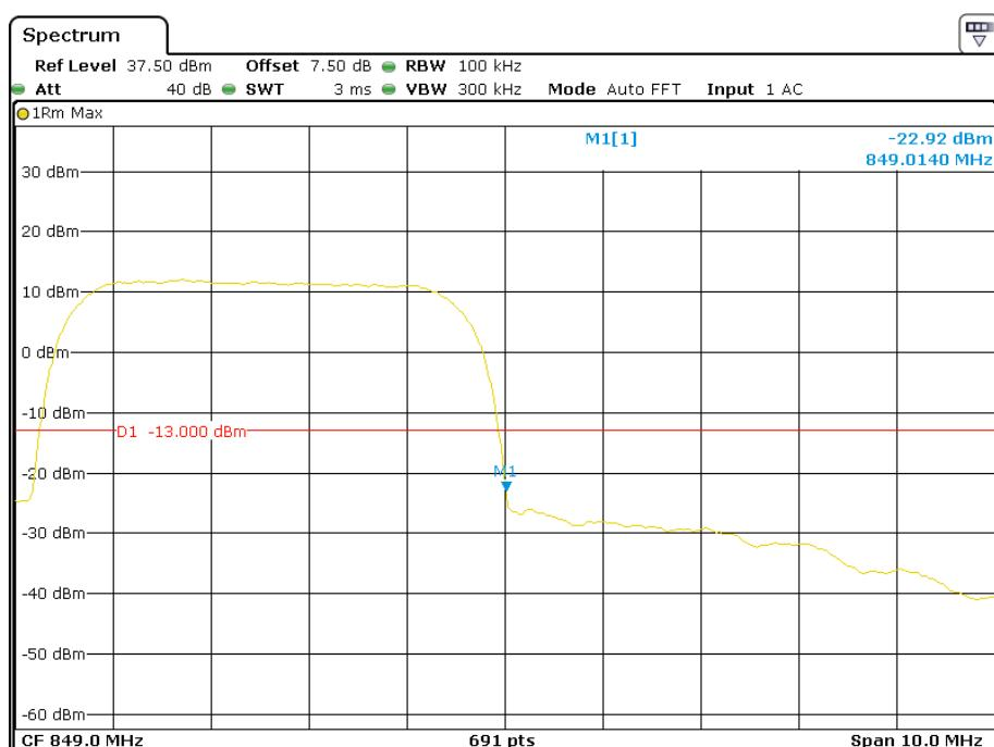
**Cellular Band, Left Band Edge for HSUPA (BPSK) Mode**
