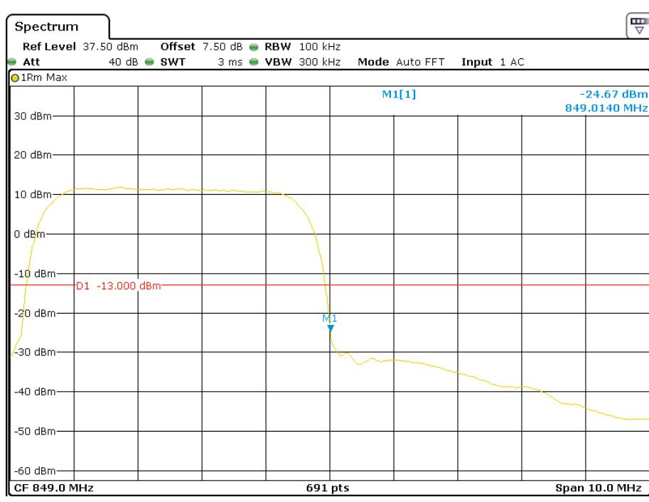
**Cellular Band, Left Band Edge for HSDPA (16QAM) Mode**
