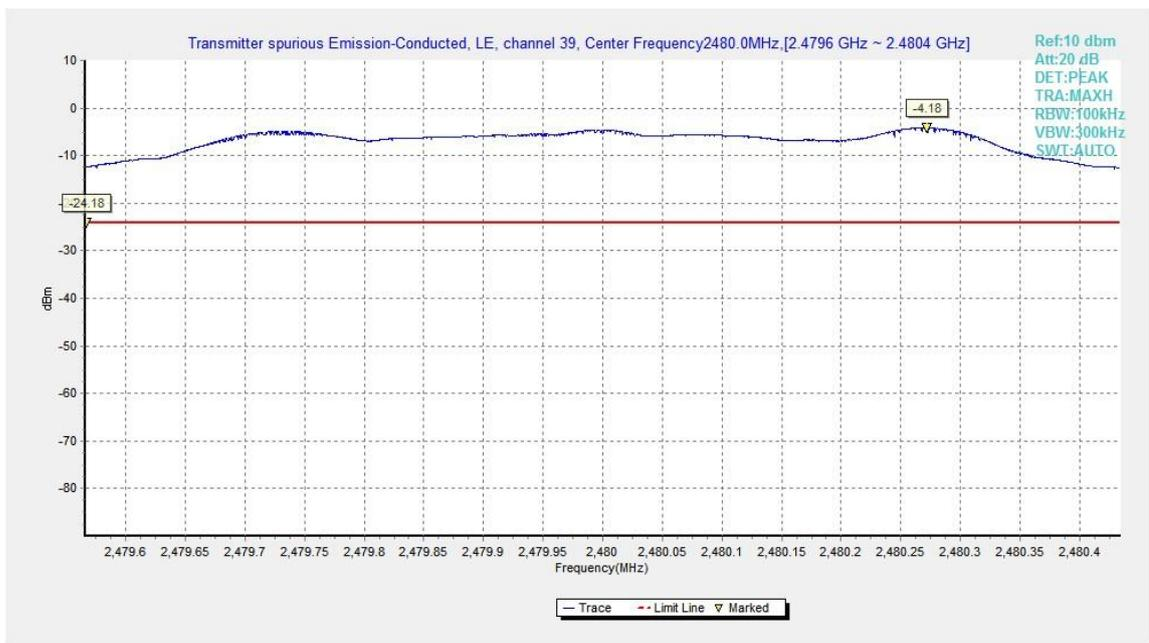
**Fig.15.** Transmitter Spurious Emission - Conducted: GFSK, 2480 MHz
