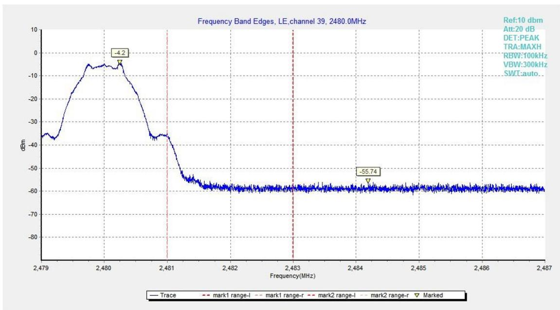
**Fig.2.** Frequency Band Edges: GFSK, 2480 MHz, Hopping Off
