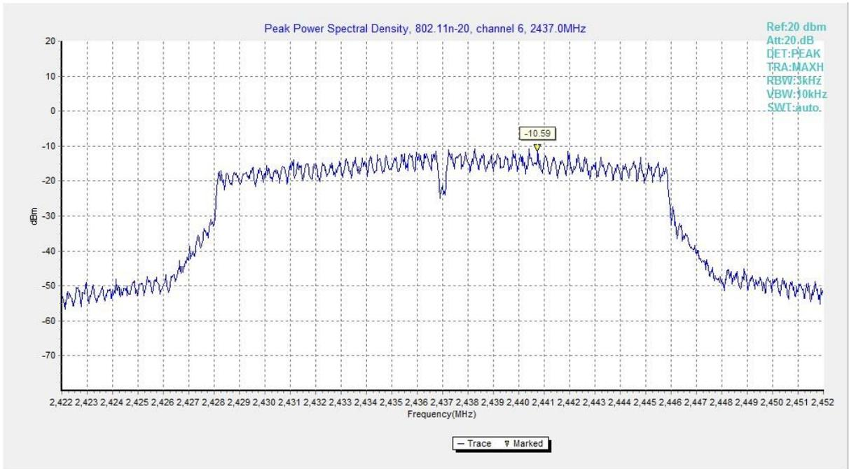
**Fig.8 Power Spectral Density (802.11n HT20, CH 6)**
