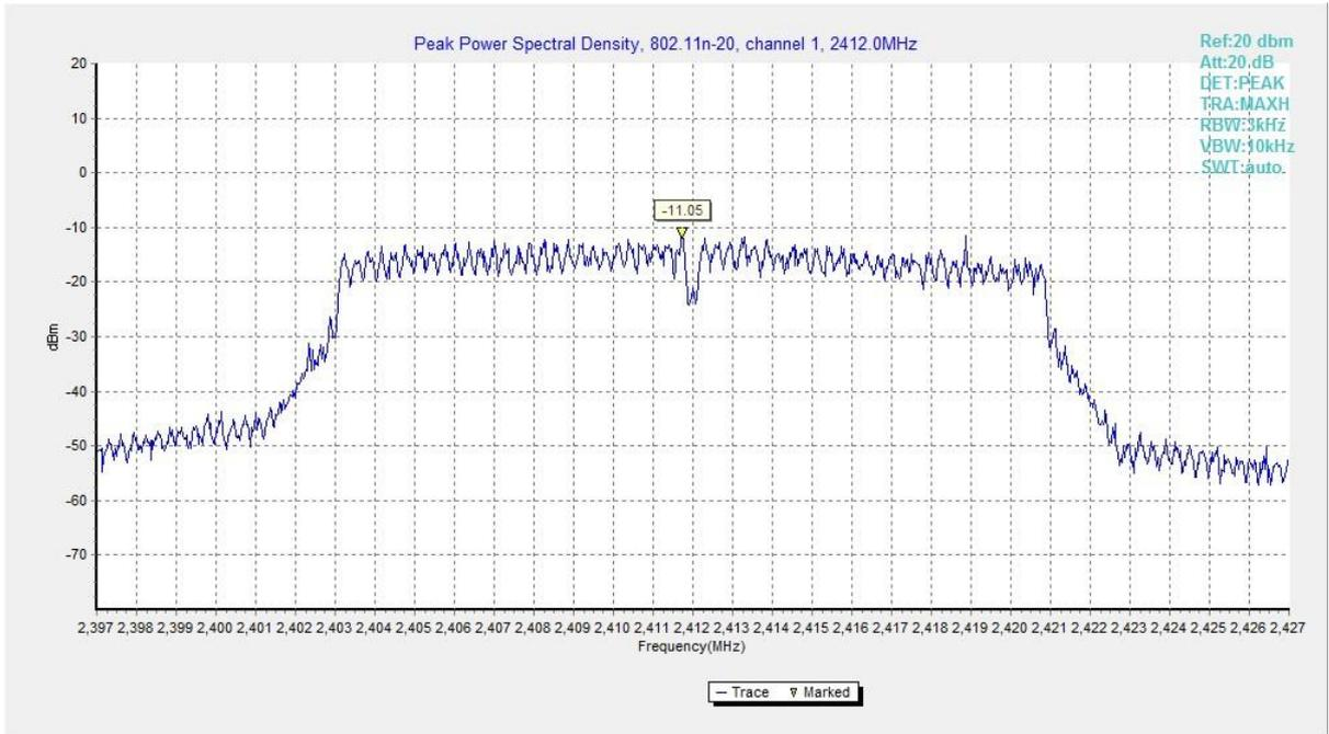
**Fig.7 Power Spectral Density (802.11n HT20, CH 1)**
