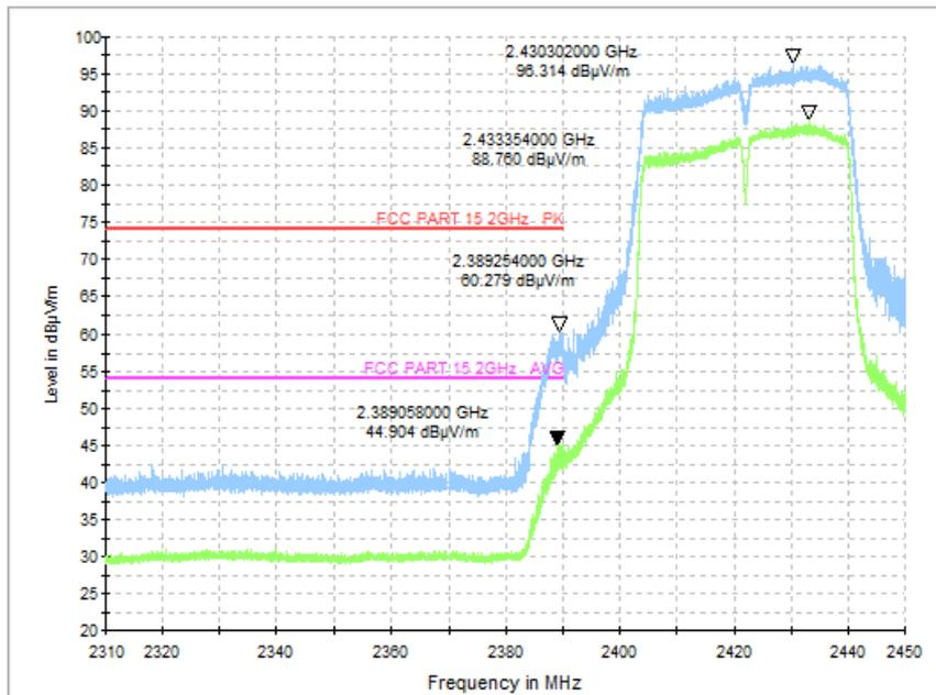
Fig.63 Radiated Restricted Band (802.11n HT40, CH3, 2.38GHz~2.45GHz)
