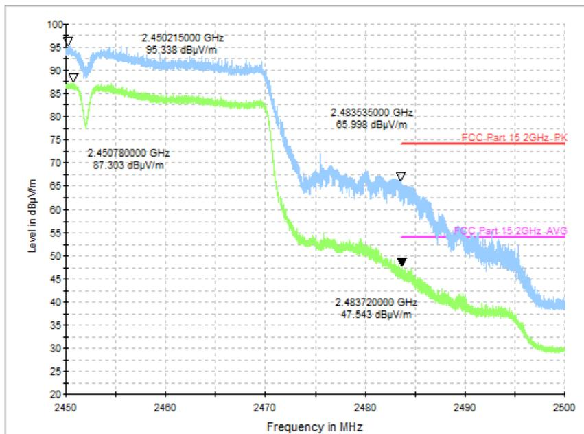
Fig.64 Radiated Restricted Band (802.11n HT40, CH9, 2.45GHz~2.5GHz)
