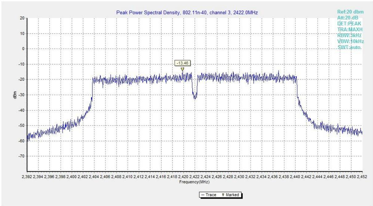
**Fig.10 Power Spectral Density (802.11n HT40, CH 3)**
