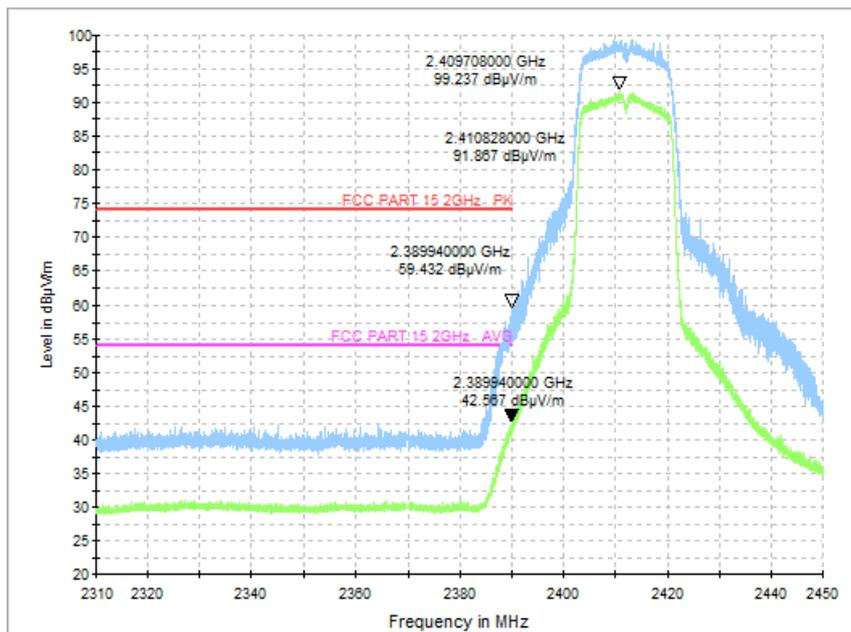
Fig.58 Radiated Restricted Band (802.11n HT20, CH1, 2.38GHz~2.45GHz)
