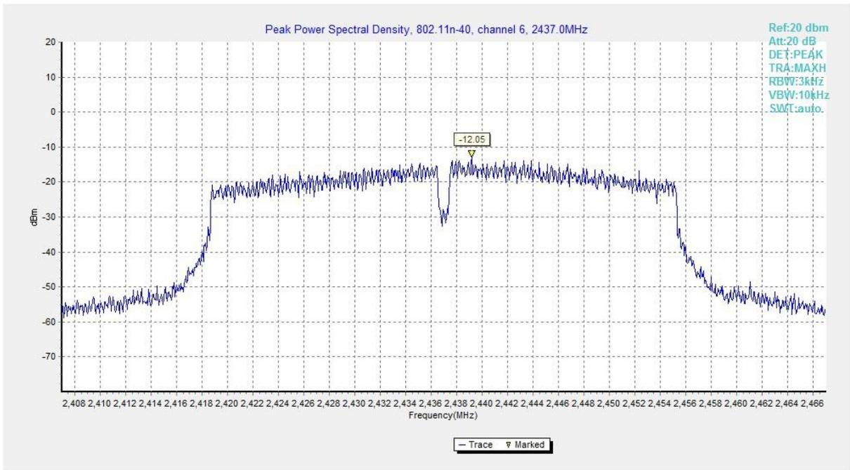
**Fig.11 Power Spectral Density (802.11n HT40, CH 6)**
