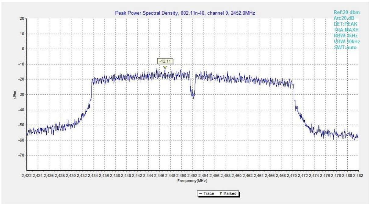
**Fig.12 Power Spectral Density (802.11n HT40, CH 9)**
