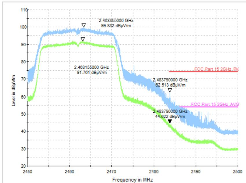
Fig.59 Radiated Restricted Band (802.11n HT20, CH11, 2.45GHz~2.5GHz)
