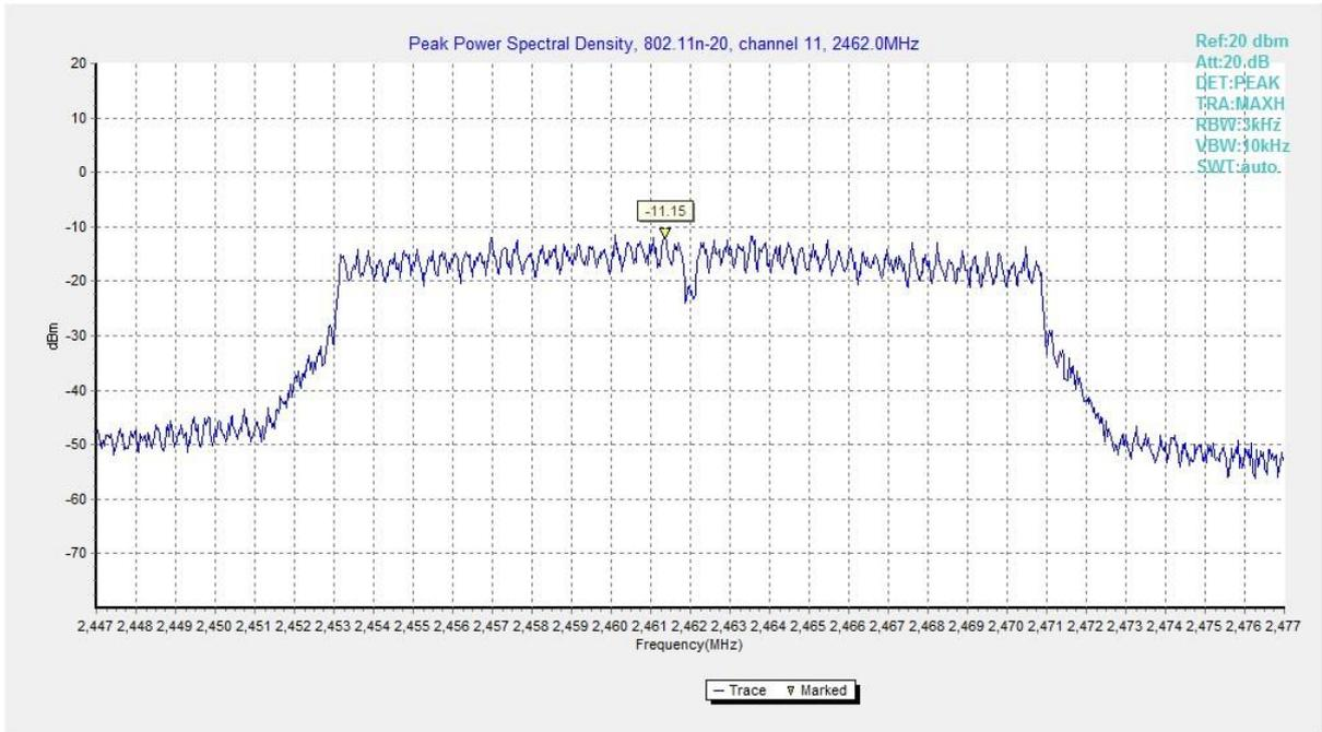
**Fig.9 Power Spectral Density (802.11n HT20, CH 11)**
