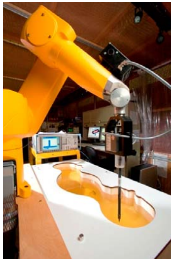
Figure 3-2 DASY4 SAR Measurement System
