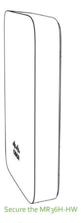
Depending on your mounting environment, you may want to secure the MR<sub>3</sub>6H-HW to its mount location. Your MR<sub>3</sub>6H-HW can be secured via security screw (Torx security screws are included).
