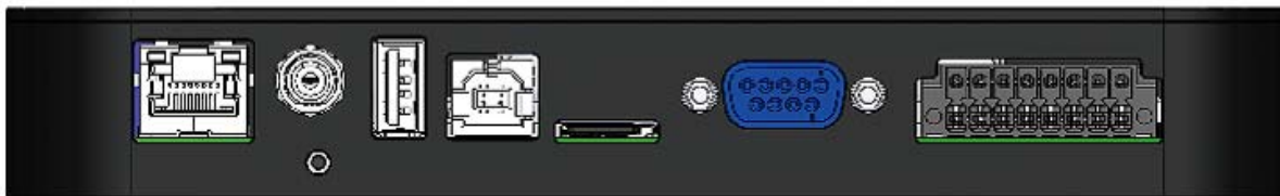
Figure 8 – Power, RS-232, USB, SDCard and LAN Connections
