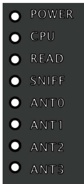
Figure 7 – ALR-F800 Front Panel Reader Diagnostic LEDs
