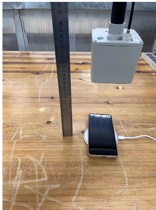
Test Position E-20cm from the edge of EUT to the geometric center of the probe
