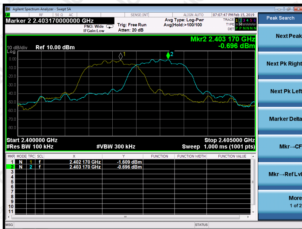
TEST PLOT FOR FREQUENCY SEPARATION ( 1Mbps )
