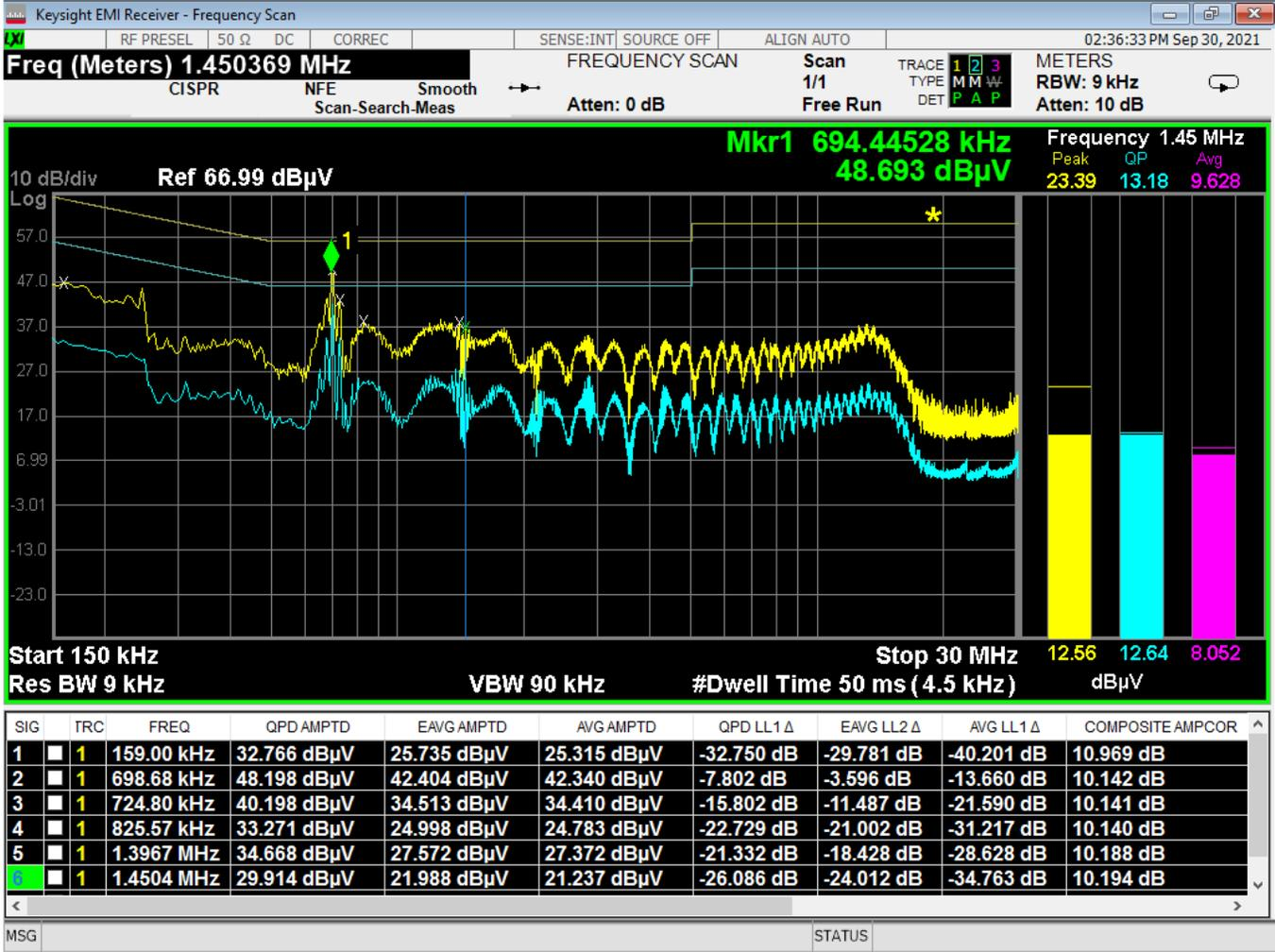
Figure 12 - Conducted Emissions Plot, Line, IDLE
