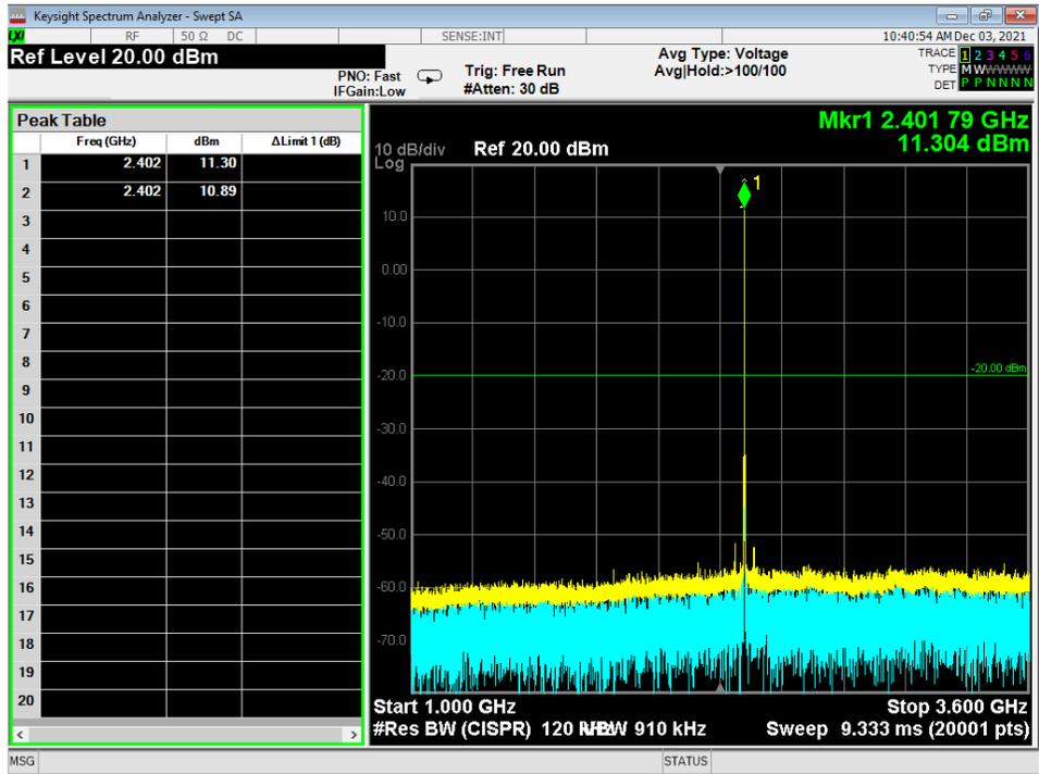
Figure 8 - Radiated Emissions Plot, BTBR, 1G – 3.6G
