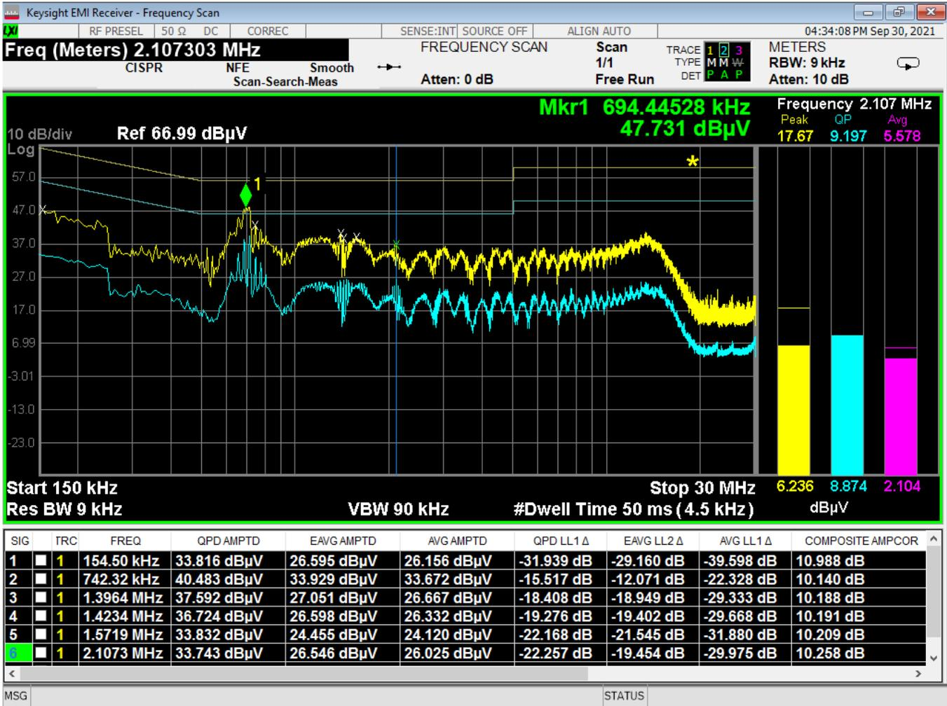
**Figure 10 - Conducted Emissions Plot, Line, TX**
