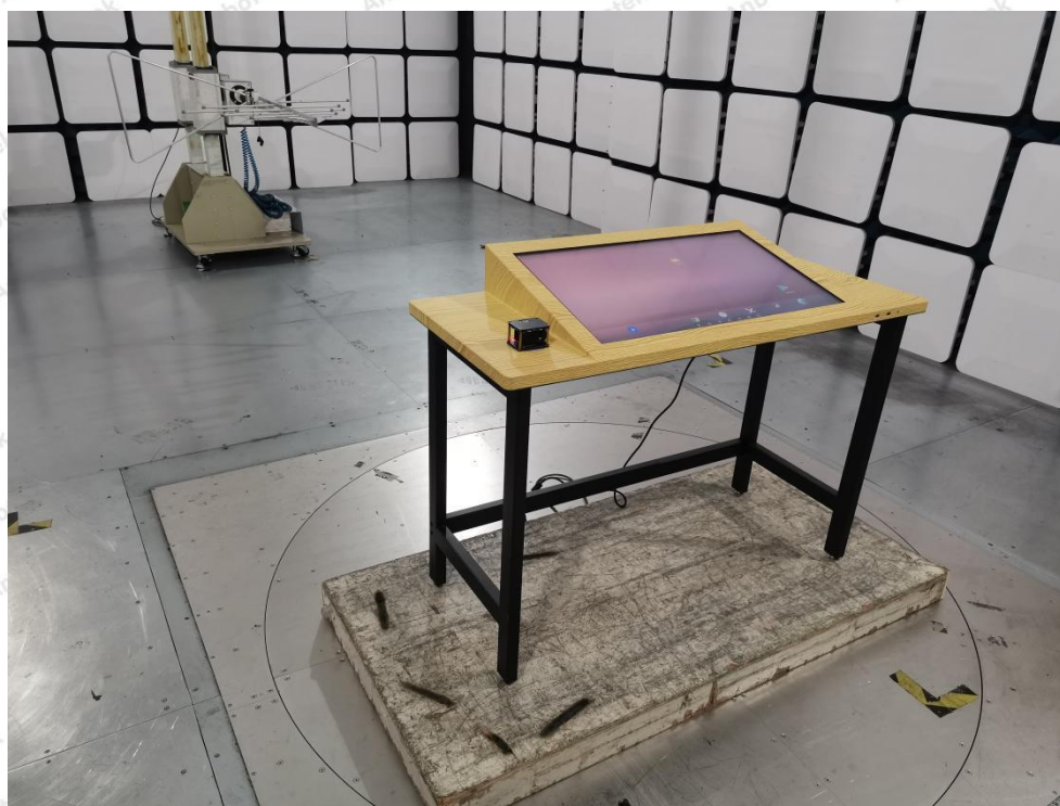
Photo of Radiation Emission Test
