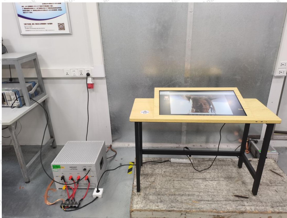
Photo of Conducted Emission Measurement
