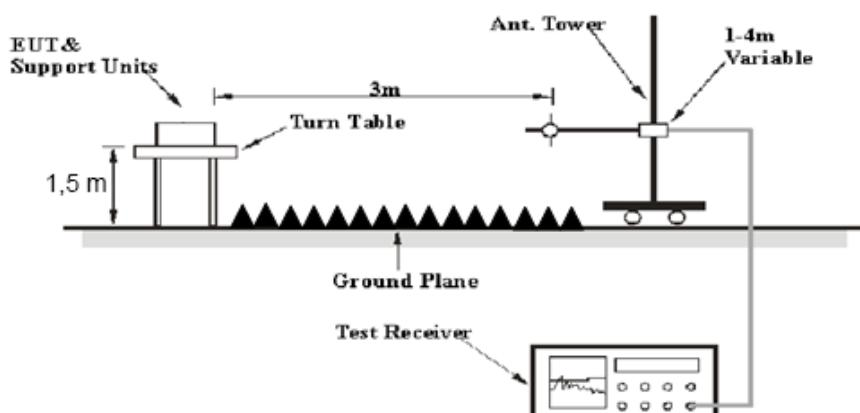
The radiated emission below 1GHz tests were performed in the 10 meters chamber test site , above 1GHz tests were performed in the 3 meters chamber test site A, using the setup accordance with the ANSI C63.10-2013. The specification used was the FCC 15.209, and FCC 15.247 limits.
