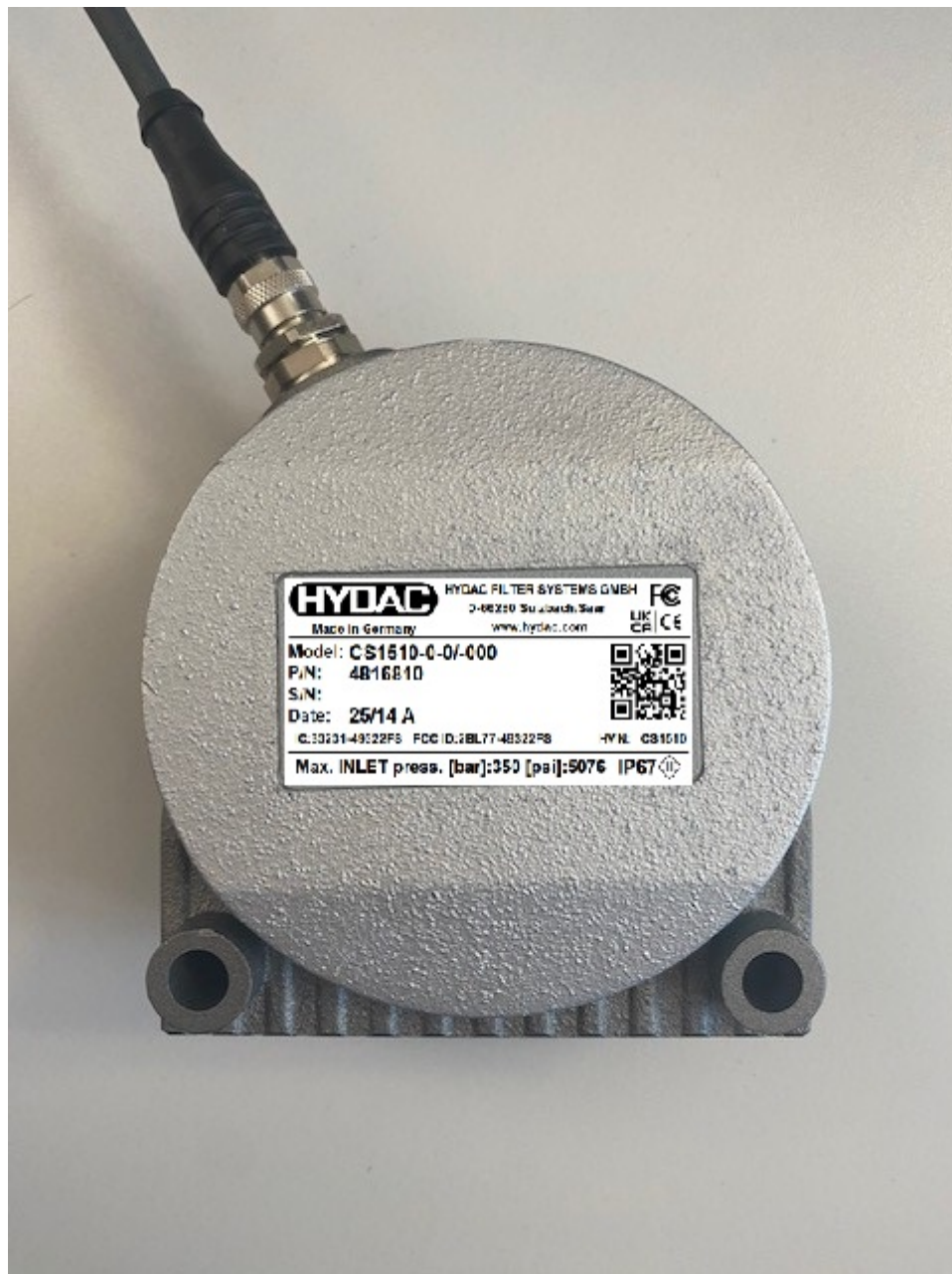
CS1500 Type Plate location (backside of CS1500)
