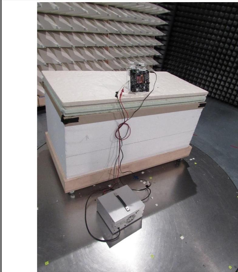
EUT Test Setup below 1 GH- Antenna 3
