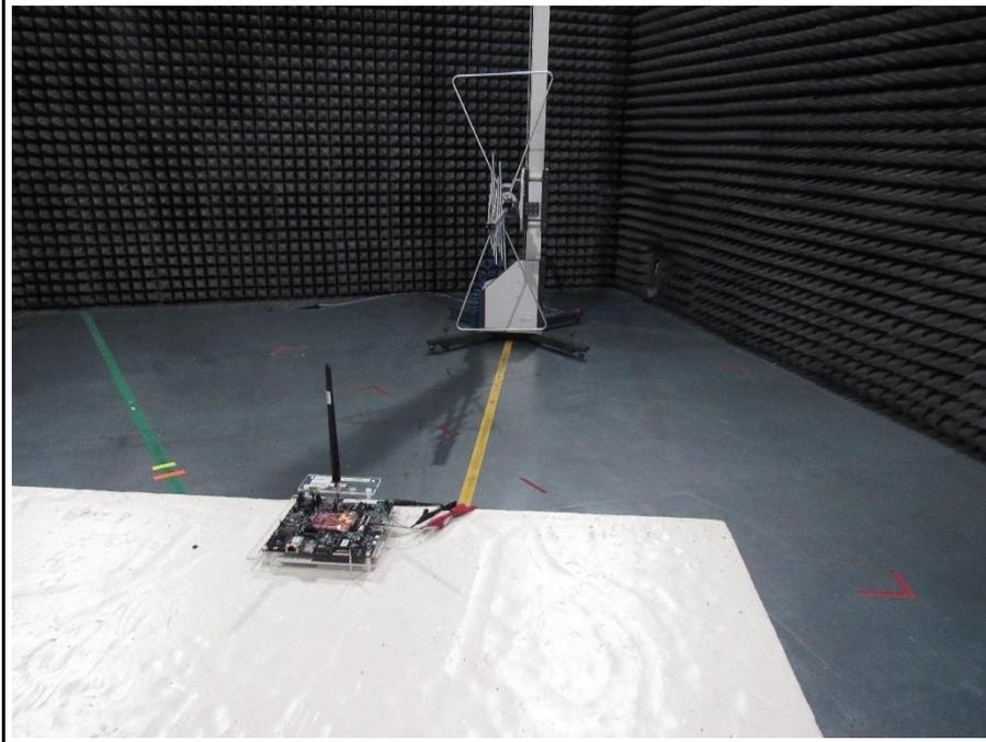
**EUT Test Setup below 1 GH- Antenna 2**
