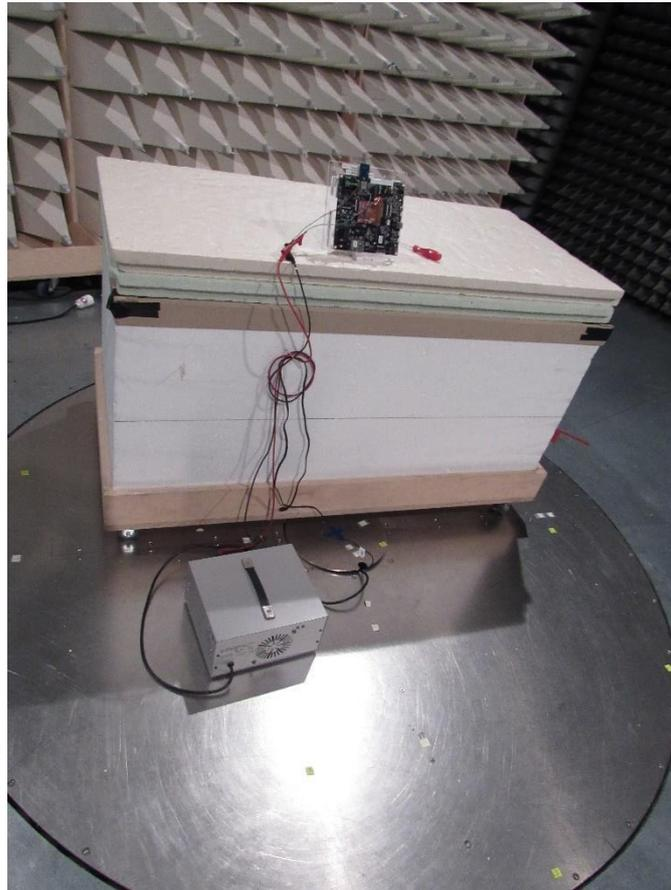
EUT Test Setup above 1 GHz-Antenna 1
