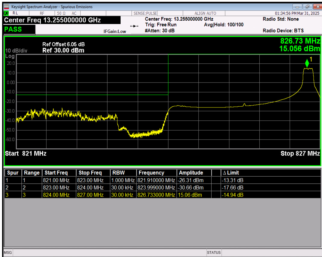
Band5 64QAM BW=3MHz Channel=20415 RB Size=15 Position=#0
