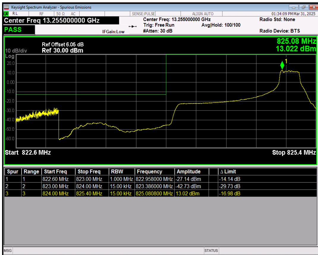
Band5 64QAM BW=1.4MHz Channel=20407 RB Size=6 Position=#0
