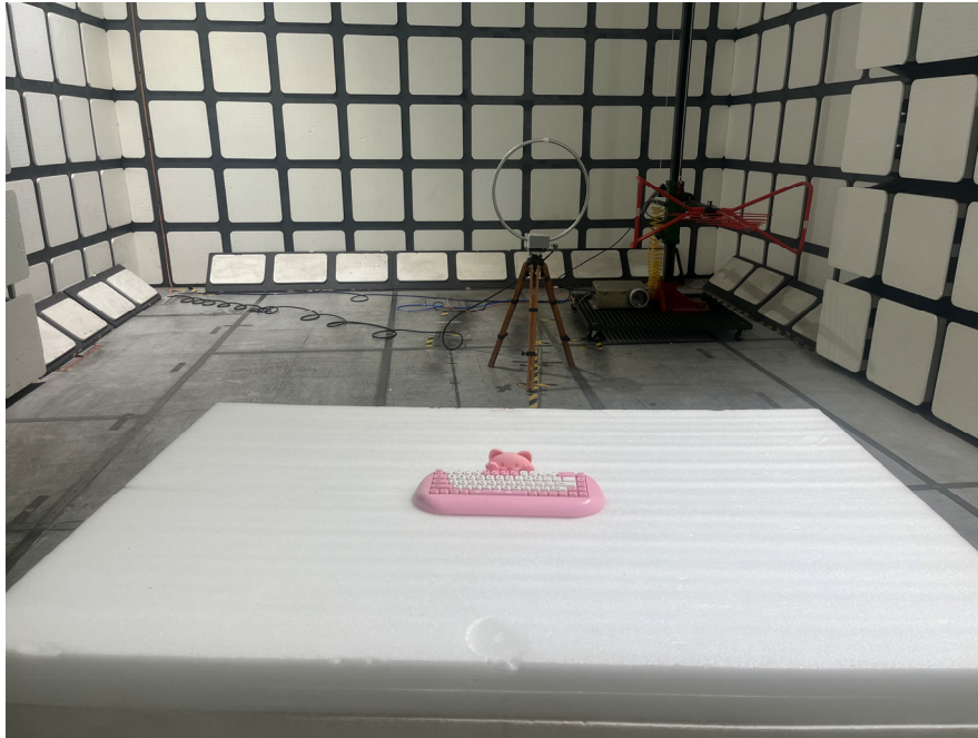
Radiated Emissions View (9 kHz- 30MHz)
