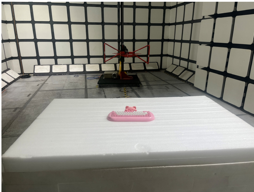
Radiated Emissions View (30 MHz- 1 GHz)
