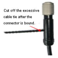
**Step 2** Fix the DC power cable connector to the PWR port, as shown in Figure 5-122. Ensure that positive and negative polarities are correct during the installation.
