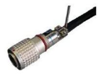
**Step 6** Pre-tighten the socket and enclosure and use the Phillips screwdriver to tighten the socket with the tightening torque no less than 1.2 N•m, as shown in Figure 5-7.
