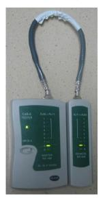
**Step 3** Gently shake the connector and repeat Step 2 to check whether the metal contact strips are in good contact with the core wires and Ethernet ports, as shown in Figure 5-87.
