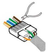
Step 5 Insert the load bar into the RJ45 connector, as shown in Figure 5-54.
