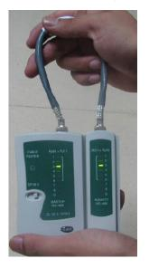
The procedure for testing a crossover cable is the same as that for testing a straight-through cable except for the sequence in which the indicators turn on, which depends on the wire connections of a crossover cable.
