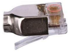
Figure 5-81 Unparallel contact strips of different heights
