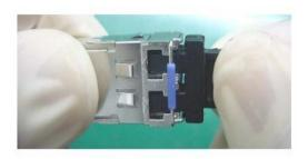
If no protective cap is available, use fibers to protect the optical module, as shown in Figure 5-171.
