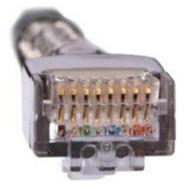
Step 2 Hold an RJ45 connector and turn it 45 °. Observe the top edges of the metal contact strips. Figure 5-81 shows an unqualified piece.
