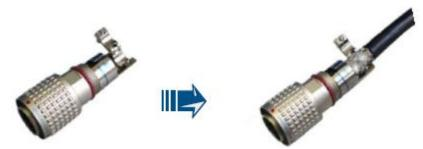
**Step 4** Use a Phillips screwdriver to tighten the crimping screw in "+" hole, rotate the connector by 180 degree, and tighten the crimping screw in "-" hole, as shown in Figure 5-5.
