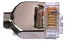
**Step 4** Check whether the contact strips and the plastic separators are well aligned and intact. If a separator is skewed and cannot be fixed, replace it with a new RJ45 connector. Figure 5-83 shows an unqualified piece.
