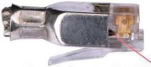
Not in good contact with the edge of the RJ45 trough
