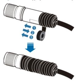
Figure 5-21 Wrapping PVC insulation tape
