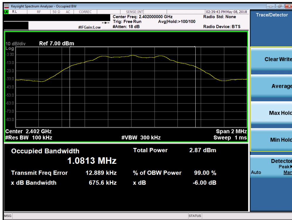
Plot 7-1. 6dB Bandwidth Plot (Bluetooth (LE), 1Mbps – Ch. 0)
