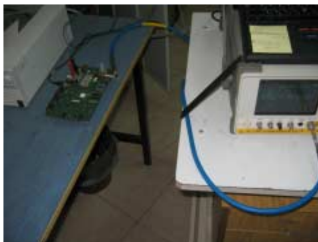
Photograph 7.2.2 Occupied bandwidth test setup
