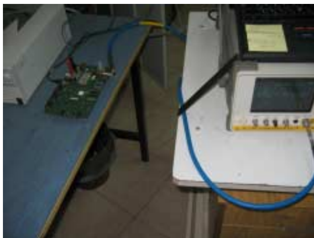
Photograph 7.1.2 Peak output power test setup
