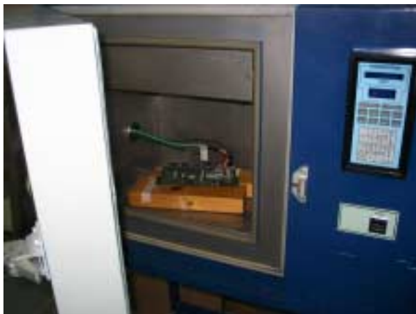
Photograph 7.5.1 Frequency stability test setup
