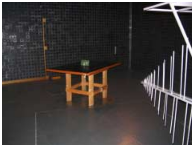
Photograph 9.2.1 Setup for radiated emission measurements, below 1 GHz
