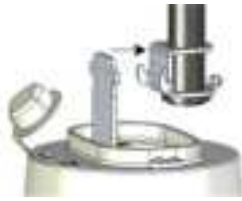
Figure 7: Hook Unit on Hanger
