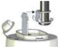
Figure 35: Hook Unit on Hanger
