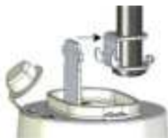
Figure 17: Hook Unit on Hanger
