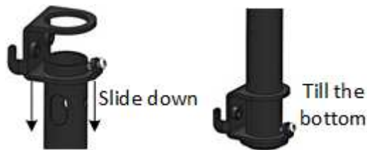
Figure 4: Slide Hanger onto Pole
