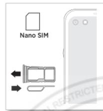
**1** Insert the SIM tool into the tray hole to pop out the tray.
