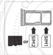
**2** Insert the SIM card(s) with the gold contacts down, then gently push the tray into the slot.
