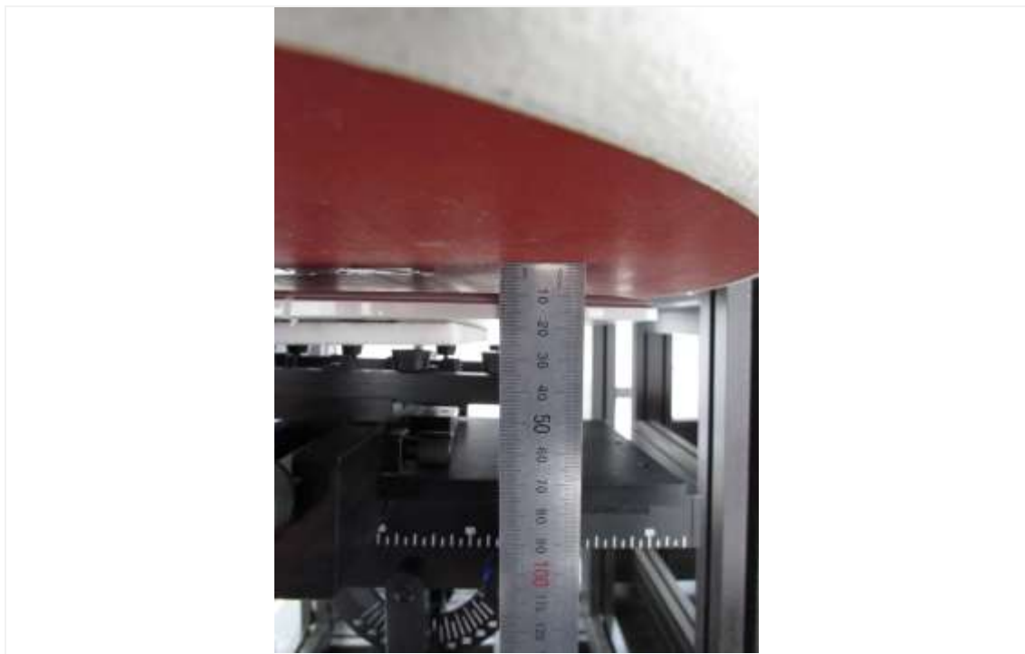
Distance of 9 mm from the EUT (WLAN ANT.2)
