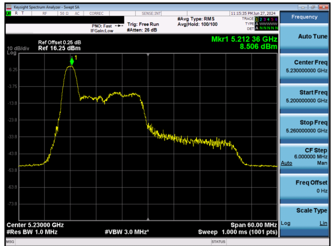
Plot 7-188. PSD Antenna WF2 (40MHz BW 11ax Index 0 - RU26 - Ch.46)
