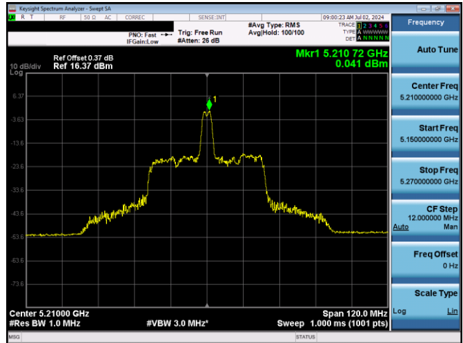
Plot 7-178. ISSED PSD Antenna WF5T (80MHz BW 11ax Index 18 - RU26 - Ch.42)
