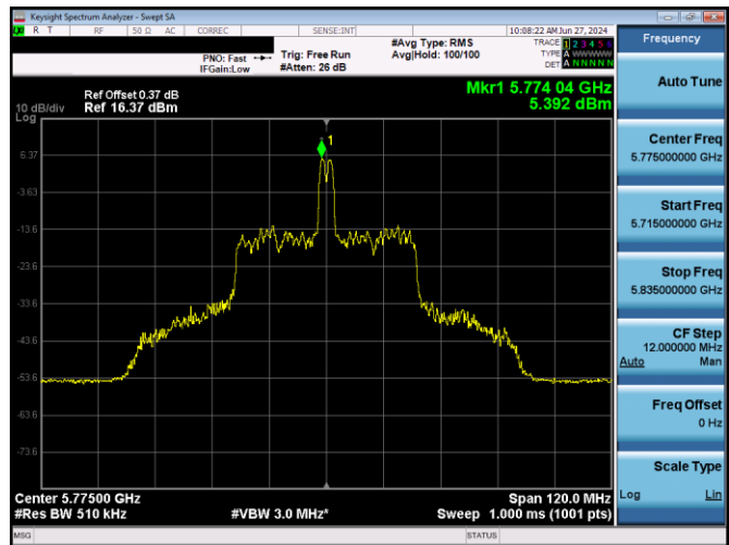
Plot 7-166. PSD Antenna WF5T (80MHz BW 11ax Index 18 - RU26 - Ch.155)
