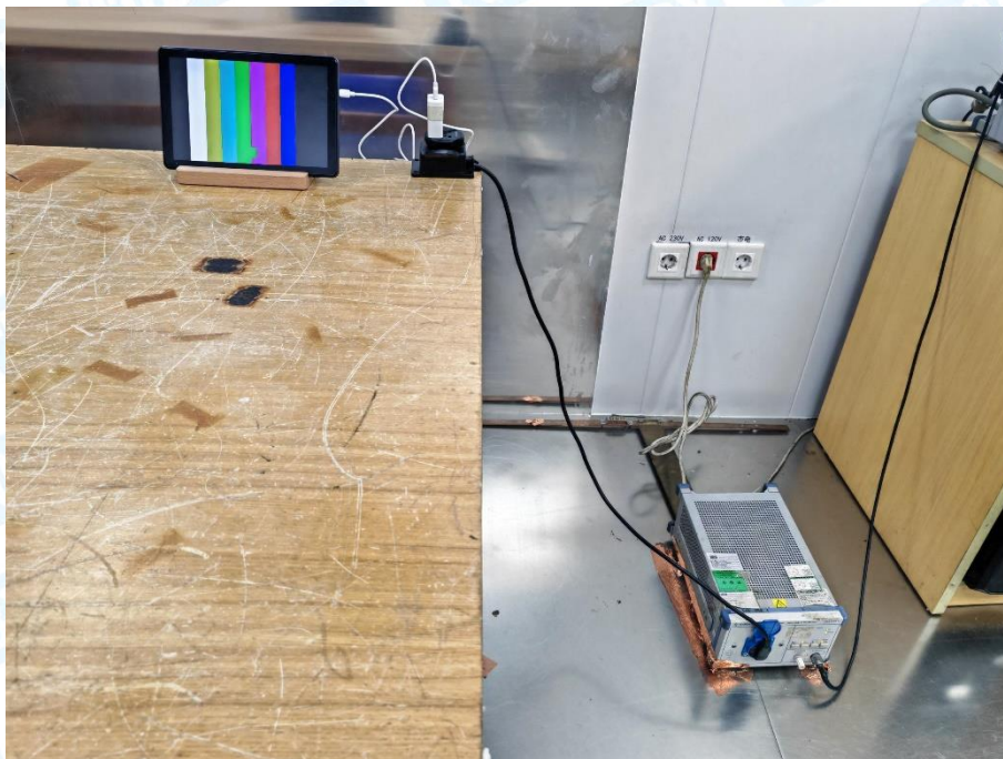
Photo of Setup for Conducted Emission
