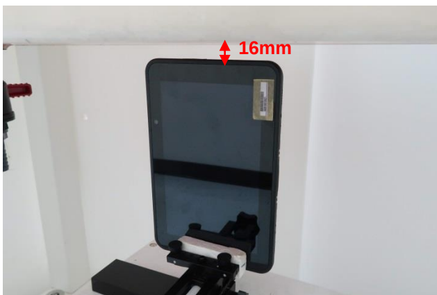
Edge4, Test Separation 16 mm
