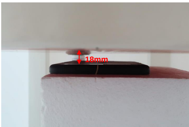
Bottom Face, Test Separation 18 mm
