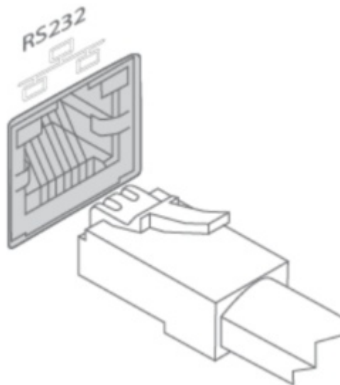
Figure 3: Connecting the interlock cable to the ZBAMB9012 controller
