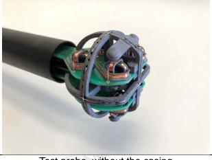
Test probe, without the casing
