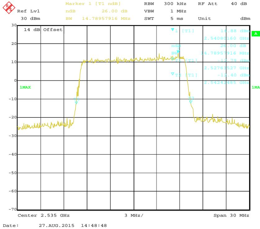
**16-QAM (15.0 MHz) - 26 dB Bandwidth, Middle channel**
