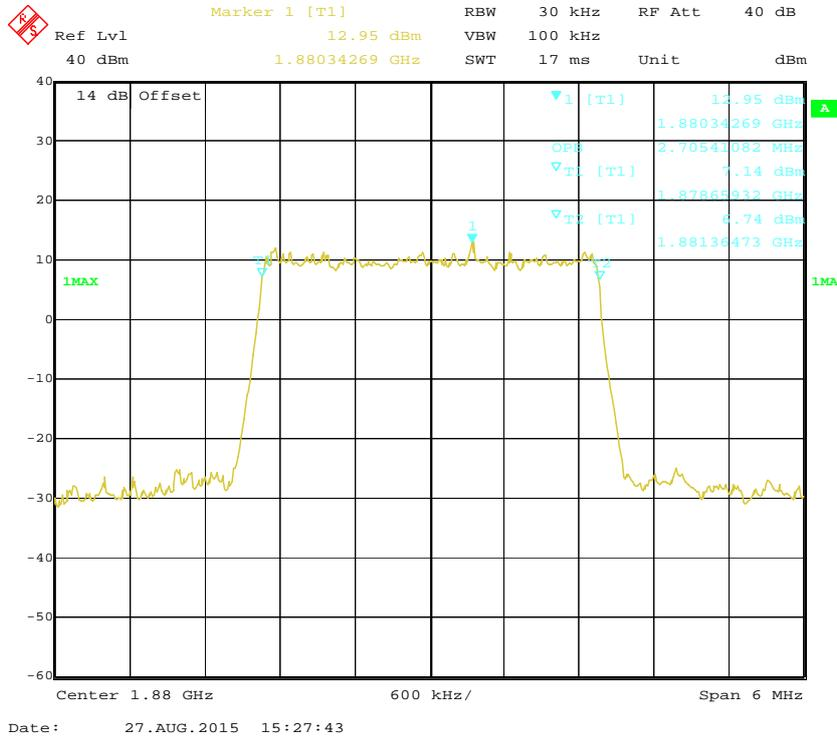
**16-QAM (3.0 MHz) - 99% Occupied Bandwidth, Middle channel**
