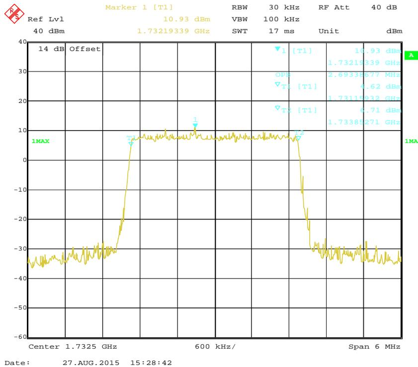
**QPSK (5.0 MHz) - 99% Occupied Bandwidth, Middle channel**
