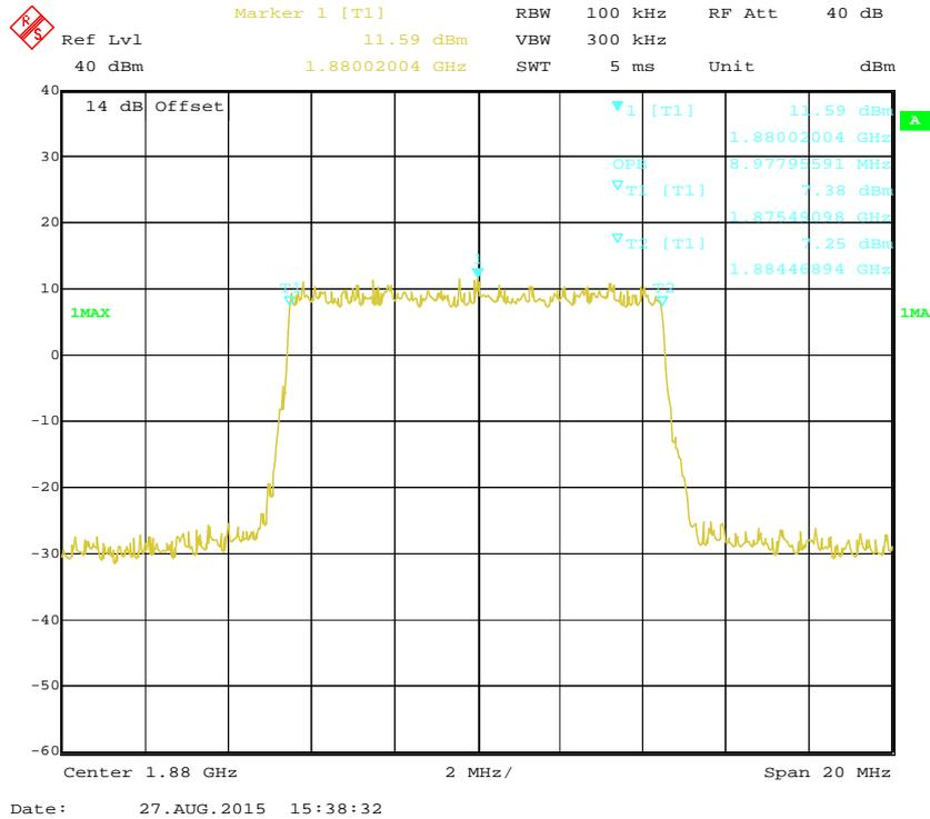
**16-QAM (10.0 MHz) - 99% Occupied Bandwidth, Middle channel**
