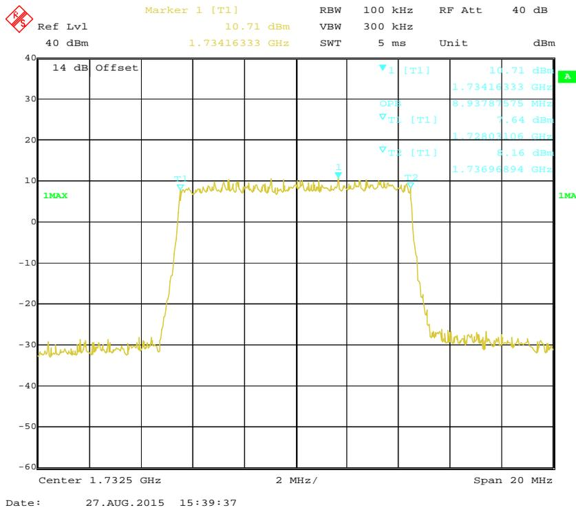
**QPSK (15.0 MHz) - 99% Occupied Bandwidth, Middle channel**
