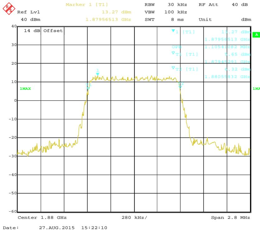
**QPSK (3.0 MHz) - 99% Occupied Bandwidth, Middle channel**
