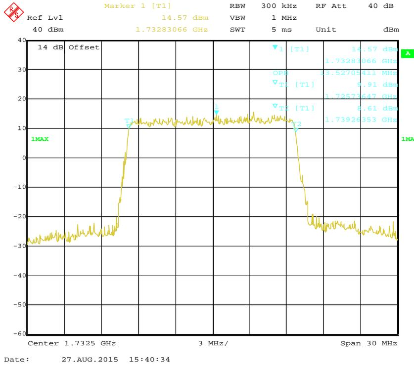
**16-QAM (15.0 MHz) - 99% Occupied Bandwidth, Middle channel**
