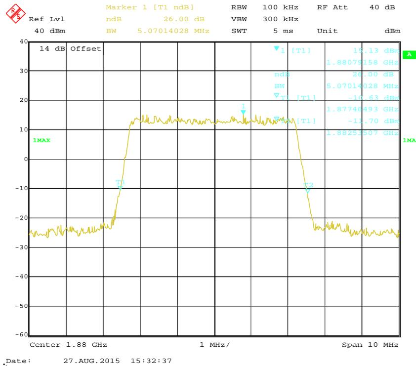
**QPSK (5.0 MHz) - 26 dB Bandwidth, Middle channel**
