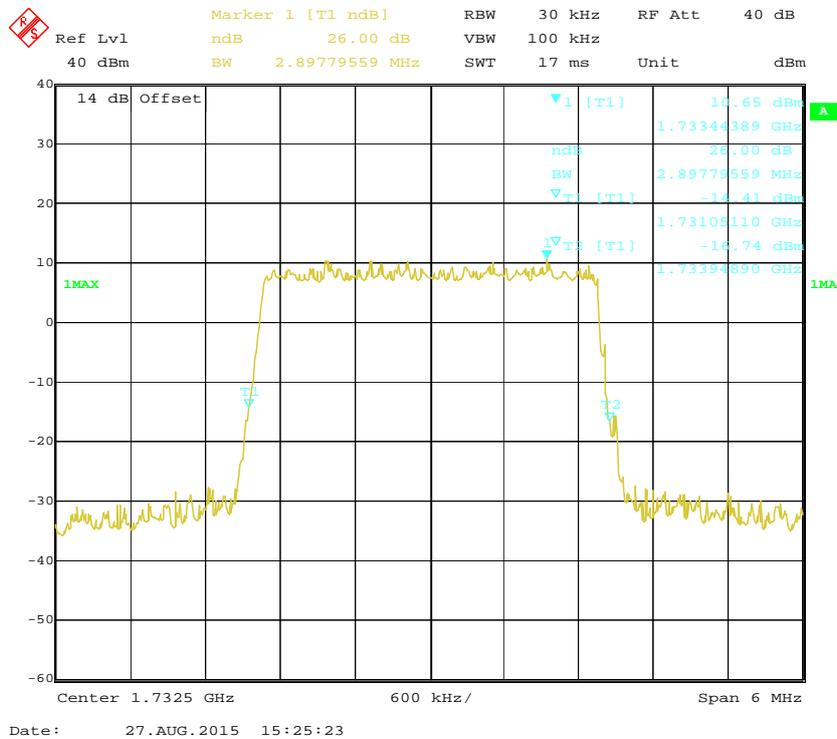
**QPSK (5.0 MHz) - 26 dB Bandwidth, Middle channel**
