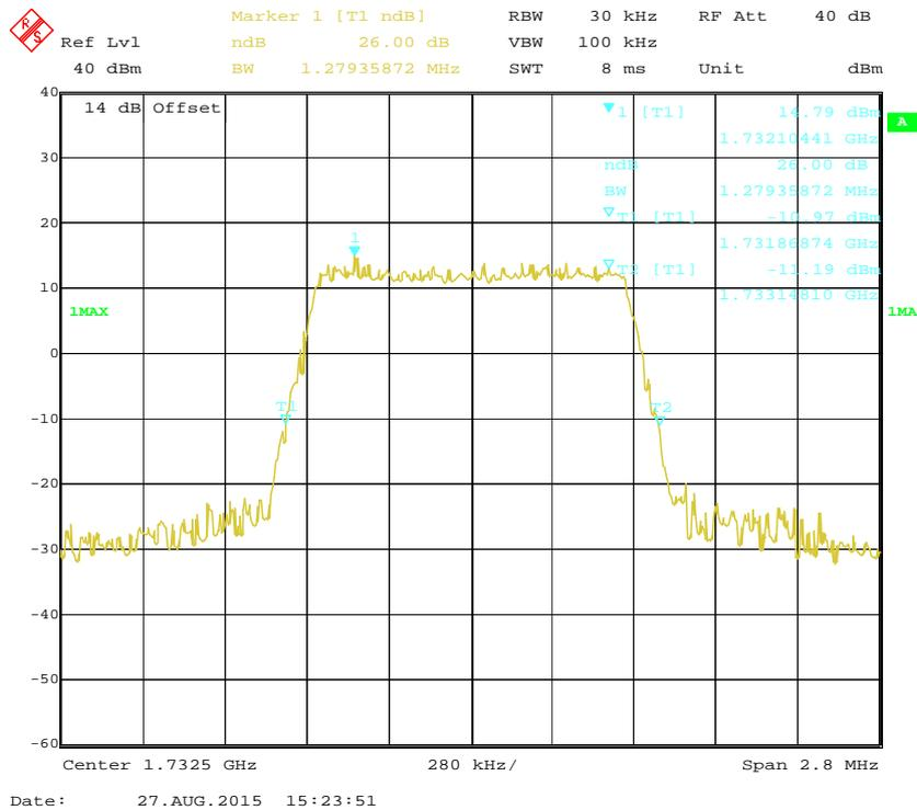
**QPSK (3.0 MHz) - 26 dB Bandwidth, Middle channel**
