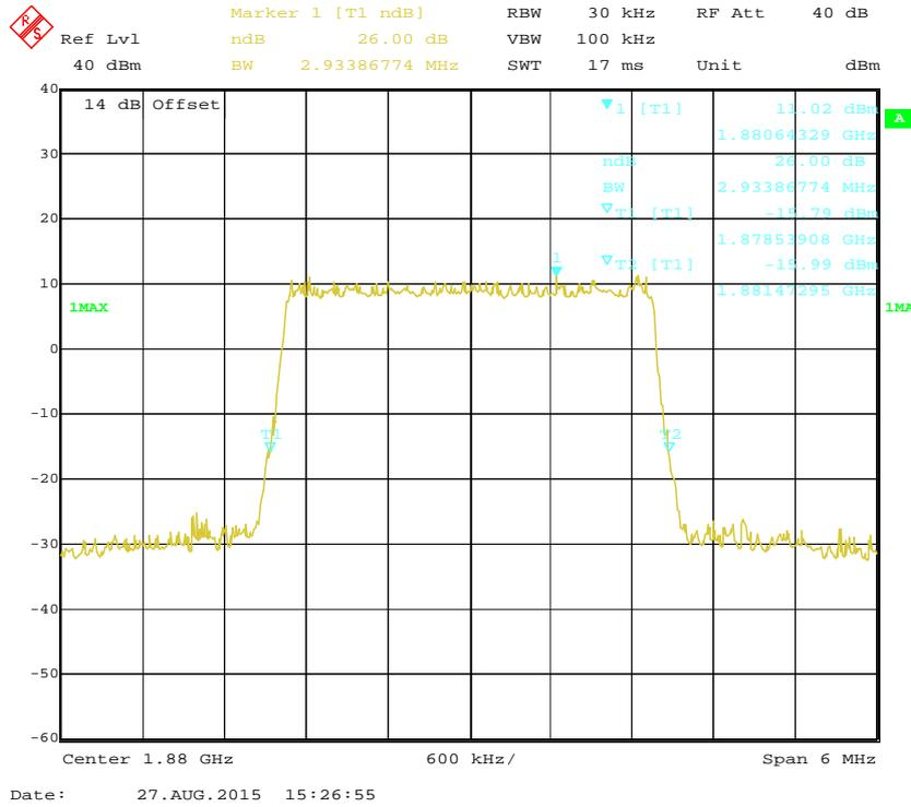
**16-QAM (3.0 MHz) - 26 dB Bandwidth, Middle channel**
