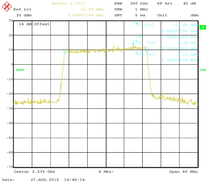
**16-QAM (20.0 MHz) - 99% Occupied Bandwidth, Middle channel**
