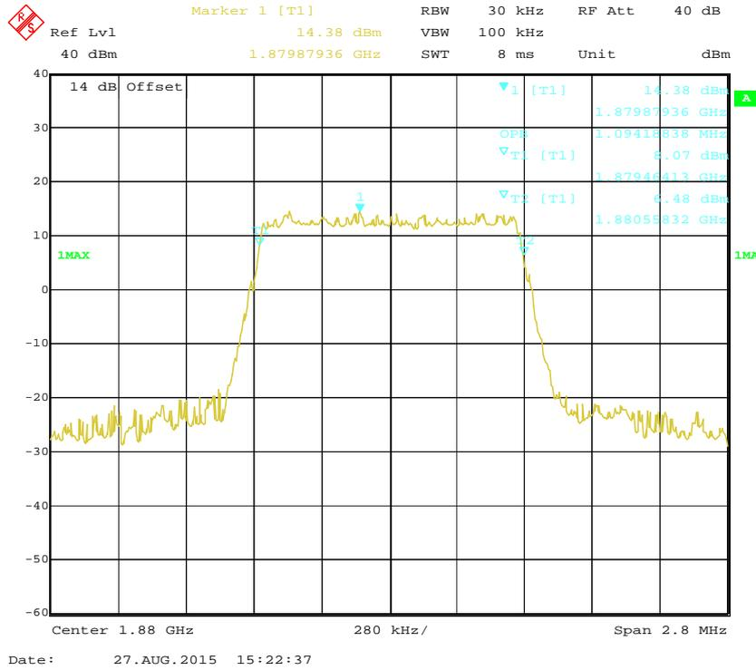
**16-QAM (1.4 MHz) - 99% Occupied Bandwidth, Middle channel**
