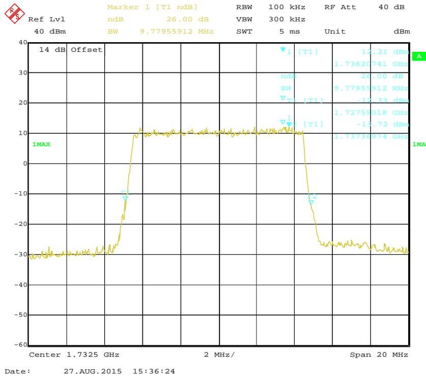
**16-QAM (10.0 MHz) - 26 dB Bandwidth, Middle channel**
