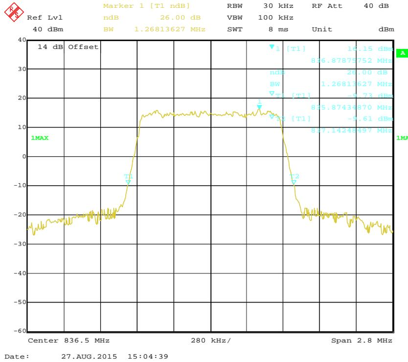
**16-QAM (1.4 MHz) - 26 dB Bandwidth, Middle channel**
