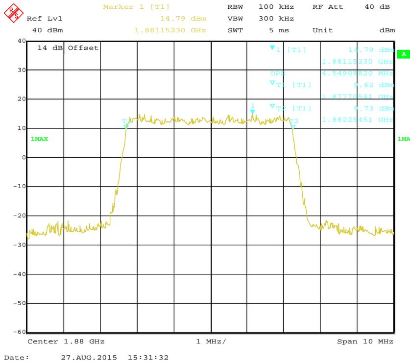
**16-QAM (5.0 MHz) - 99% Occupied Bandwidth, Middle channel**
