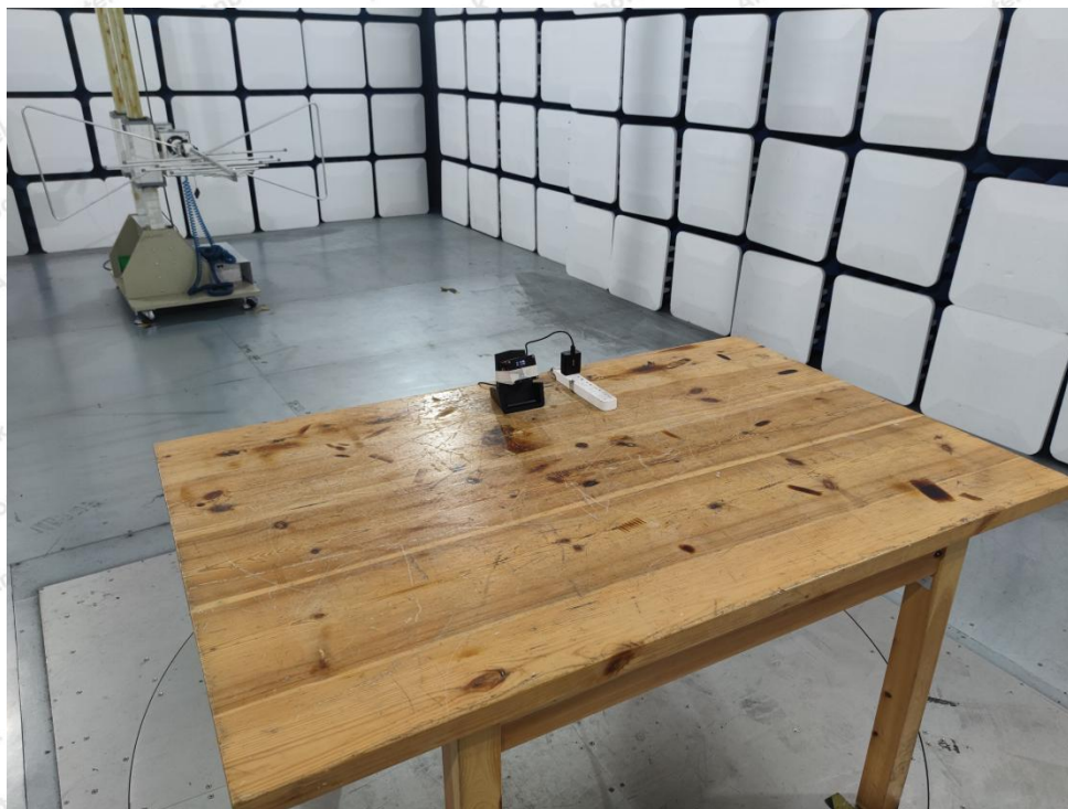
Photo of Radiation Emission Test
