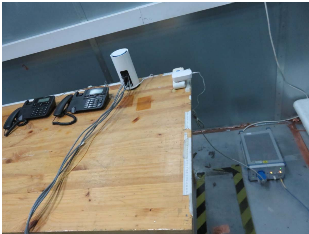
Picture 2 Conducted Emission Test Setup
