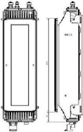
Figure 2 - AirSynergy with front sector antenna
