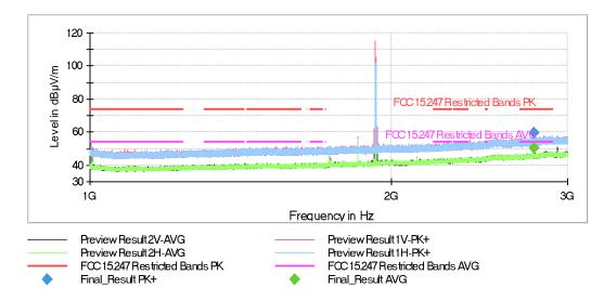
The peak above the limit is the carrier frequency DECT 1925 MHz (1928.448 MHz).
