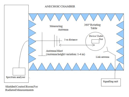
Radiated measurements between 1 GHz and 10 GHz.
