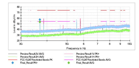
Peaks above the limit are due to the DECT technology and no radiated spurious limit applies to it.
