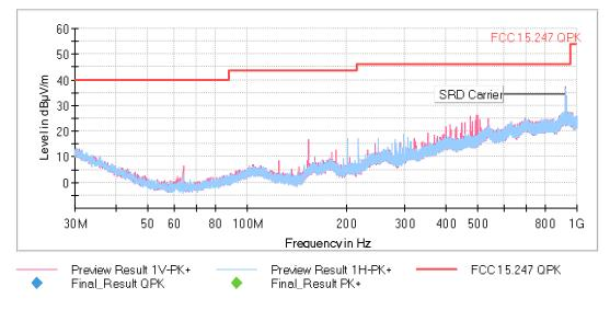
The highest peak is the carrier frequency SRD (925.5 MHz).
