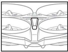
4. When fully charged vehicle light turns off.
