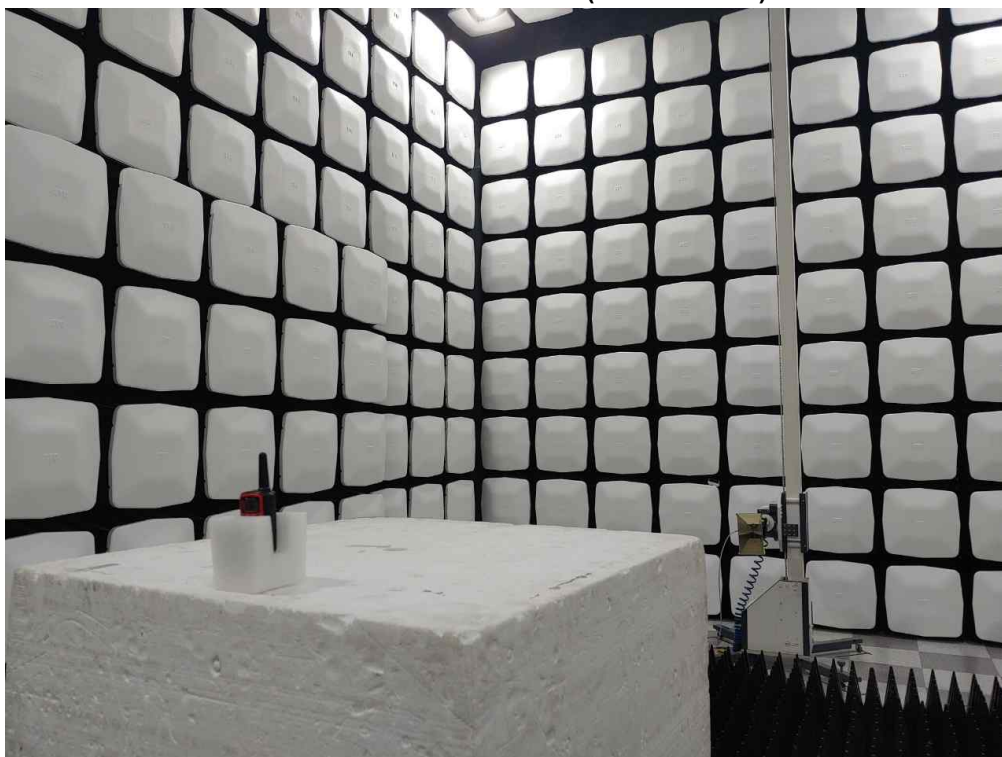
Radiated RF measurement(Above 1 GHz)
