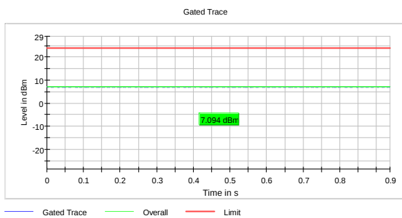
RMS Conducted Power, 5500 MHz, 802.11n, HT20, MCS0, Ant1
