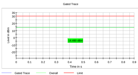
RMS Conducted Power, 5755 MHz, 802.11n, HT40, MCS0, Ant1
